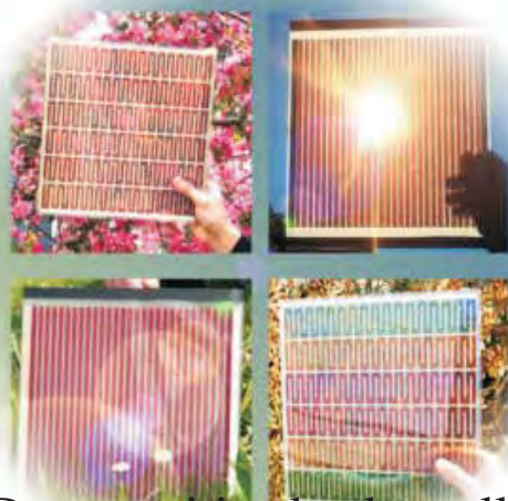
Dye-sensitized solar cells use ruthenium compounds
