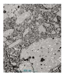
$\rightarrow$  2. Electron backscatter image of the typical microstructure of an MgO-based brick.
