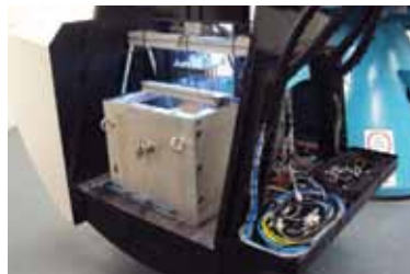
Centrifuge model: A scale model on the swing of the 150 G-ton centrifuge where 48 channels of data can be recorded during testing.
