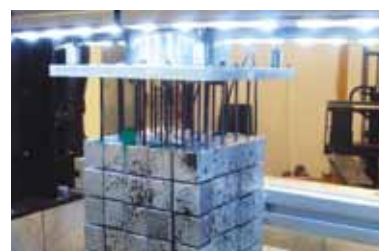
Loading model: A scale model of large-scale surcharge tests conducted along the Gautrain route.
