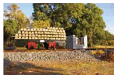
Railway line: Load tests on the section of railway line constructed for research purposes on the University of Pretoria's Research Farm.
