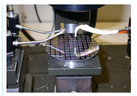
$\rightarrow$  The optical performance of new INSiAVA silicon light sources is characterised by a fibre-optic measurement probe on a micro-manipulator.
