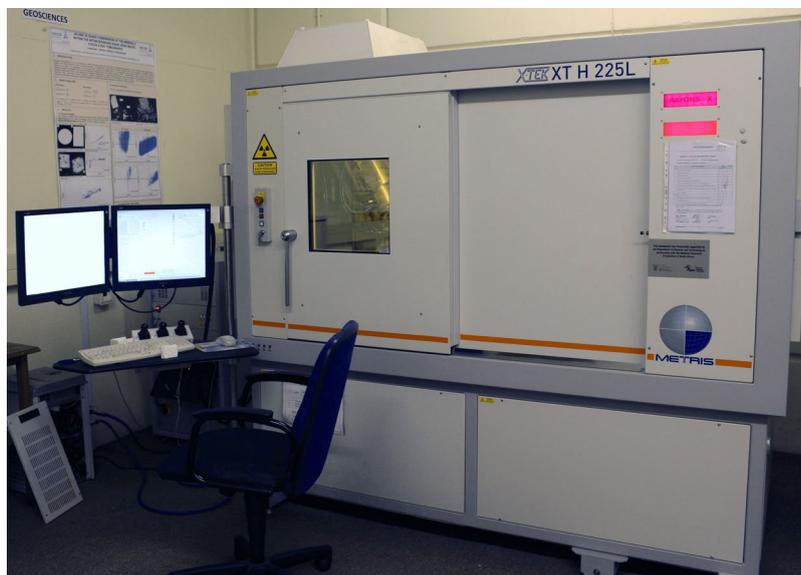
**Figure 3.** *Example at Necsca: Nikon XT H 225L industrial Computed-Tomography system.*
