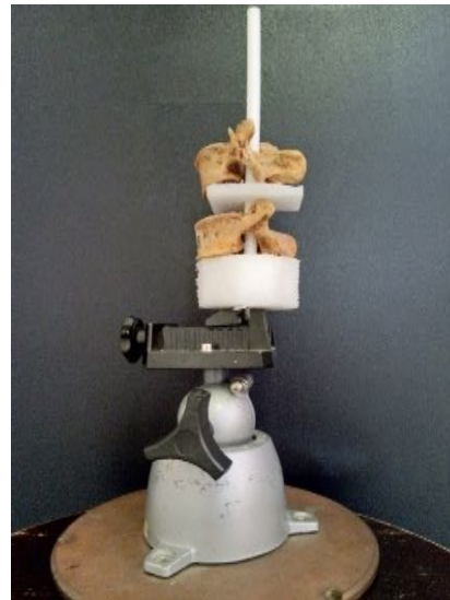
Figure 6.2: Lumbar vertebrae mounted on the stand with foam separators
