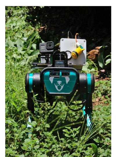
With the help of artificial intelligence, robotics and Big Data, the University, through the Department of Civil Engineering, is making use of its four-legged terrestrial robot. SmWoef is used to facilitate data collection in high-risk environments that are difficult or unsafe to access for human, or that require repetitive data collection. This is an excellent example of how robots and humans can co-exist and work together to innovate our tomorrow.
