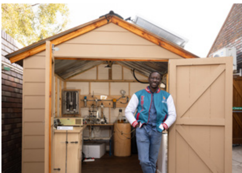
Dr Samuel Iwarere demonstrates the functioning of a simulated laboratory for the development of solar-powered plasma technology to treat contaminated water in rural communities. It includes a solar panel on the roof of the outdoor laboratory.
