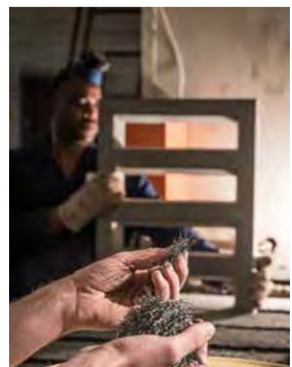
→ Steel fibres are used to reinforce the concrete.
