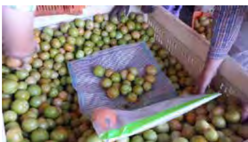
→ Installation of the pressure sensors in the half-bins.
