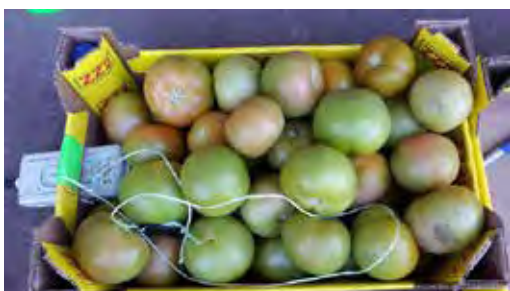
→ Installation of accelerometers on the small boxes.
