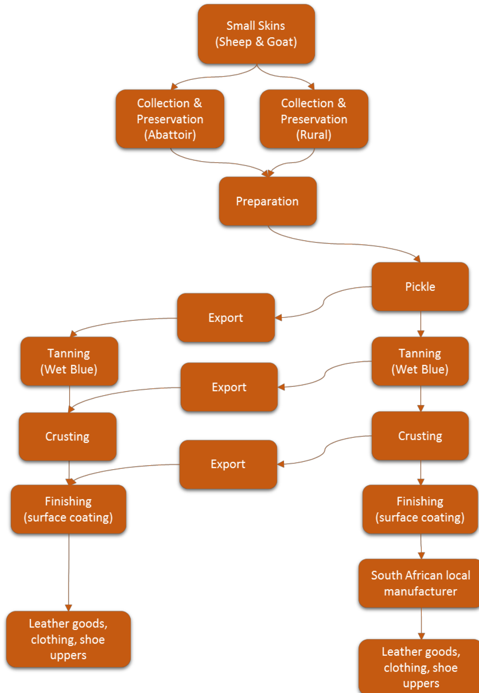
Figure 1-4 The production flow of skins through SA processing units. (Modified from UNIDO, 1991)
