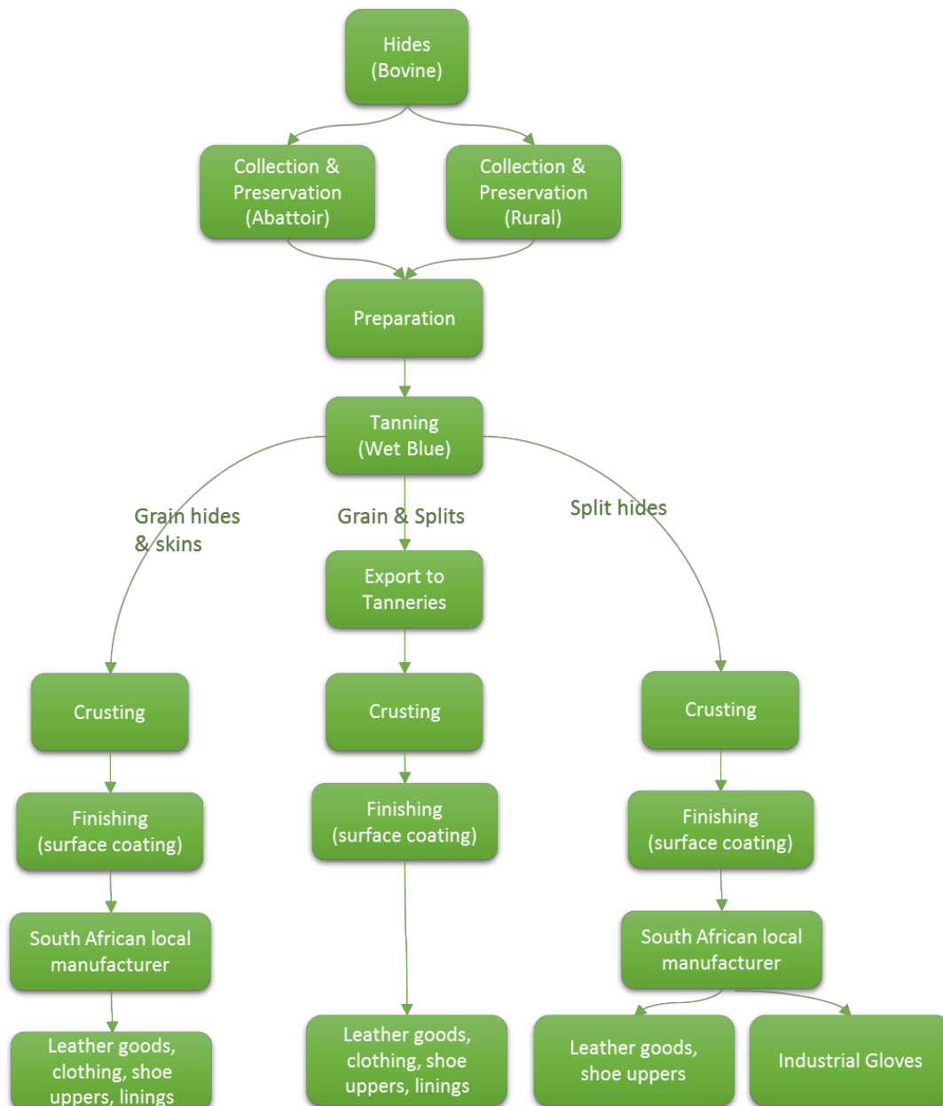
Figure 1-2 The production flow of hides through SA processing units. (Modified from UNIDO, 1991)
