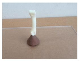
In the case where your item is not too complex and you can take the risk to cut on or very close to the surface of it, the following method might be possible. Fix the item on a cone of plasticine, imagine your item like a tree branching upward. The cavity left by the cone will eventually also act as a funnel to cast your item. If there are parts turning down, you will need to create breather tubes to the bottom, or avoid this method.
