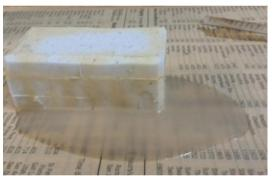
The item can then be removed from the first casting, all the time taking care not to damage the item or the mould. To cast your model, put the hollow part of the mould on a flat, level surface and mix 5-10% more material than the actual model will require.
