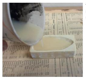
This mould you can simply put on a level surface, mix your material of choice, pour until it is level with the sides, and remove it the same way you as the original when cured.
