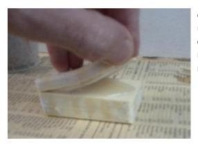
or using it again, it important to clean off all casting material from it. There are usually a thin layer of your casting material forming between the two halves of the mould, it is special important to clean this off as this can ruin following castings.
