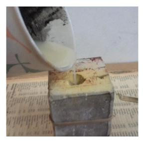
Pour the cast material slowly through the funnel, let cure, remove like the original. Your model will now have a cone shape protruding from it which you can cut off and work until smooth.
