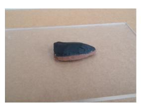
If the item you want to duplicate is flat, with no detail of any importance on one side, you can get away with a simple open mould. Simply fix the item on a flat surface (that will be the bottom of your box), making sure not to damage the original in doing so. Sticky putty or plasticine can be used for this purpose. Build a box around your item, leaving enough room to ensure a sturdy mould, and high enough to cover the object.
