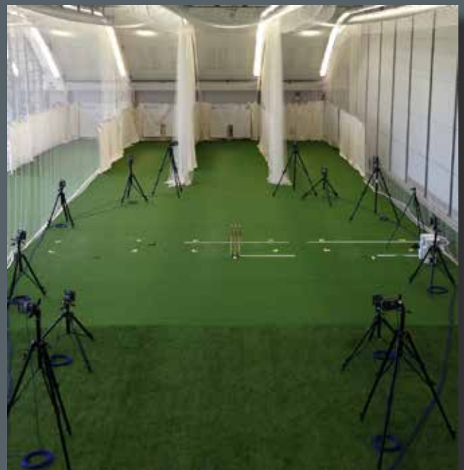
Three-dimensional motion capture setup in the Cricket South Africa Centre of Excellence at the University of Pretoria
