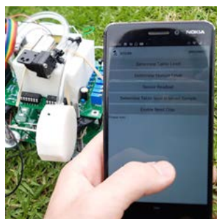
An e-nose for monitoring the Amitraz concentration in a cattle dip tank (by Archibald Rohde)
