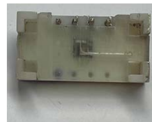
A CMOS integrated circuit in an additively manufactured microfluidic device (by Abraham Salom)
