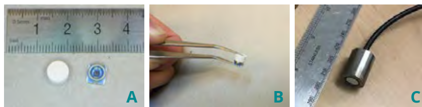
→ Figure 1A: Ceramic filter and pressure sensor; 1B: Filter-sensor assembly; and 1C: The completed tensiometer.
