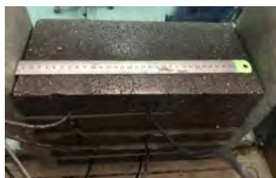
→ Figure 2: Clay slab formed by compressing clay gratings to impose artificial fissuring to allow rapid swelling in the assembly of the centrifuge model. The slabs are instrumented with moisture content and suction probes.
