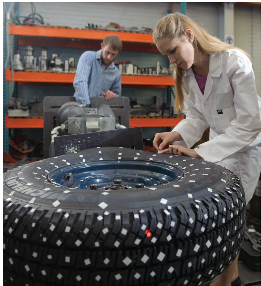
➔ Taking optical measurements on structures with complex deformation modes.
