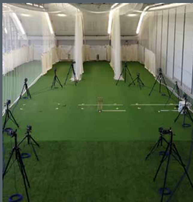
Three-dimensional motion capture setup in the Cricket South Africa Centre of Excellence at the University of Pretoria
