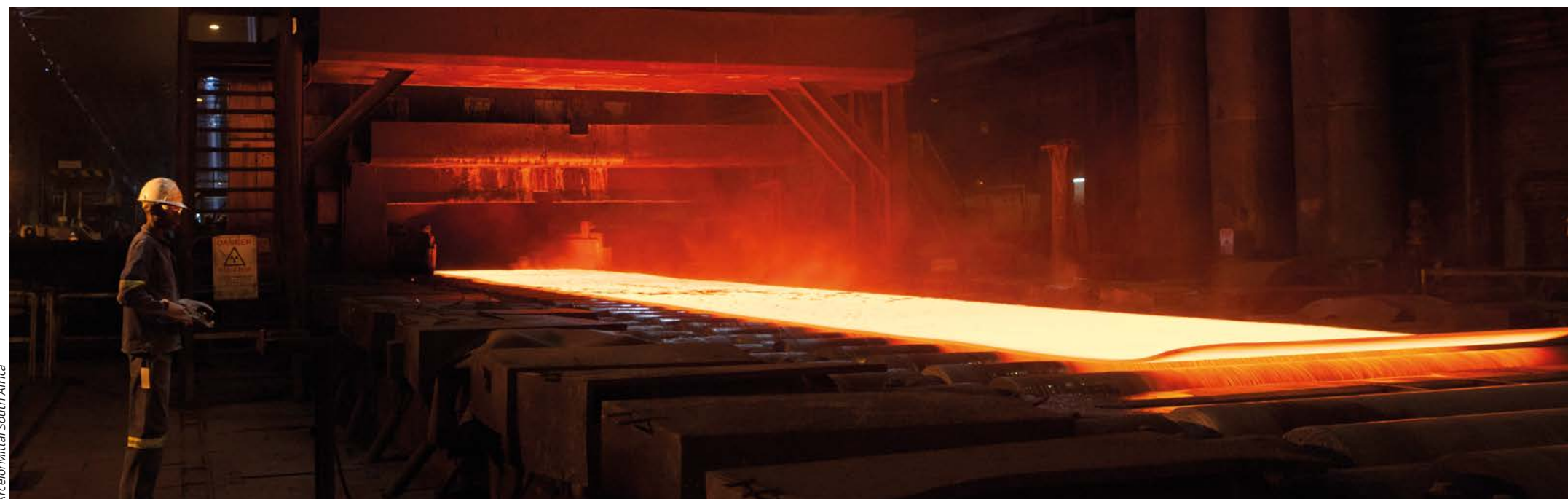
Plate mill operator about to measure the thickness of the red-hot plate rolled from an input slab.
