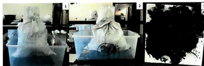
Figure 2: The fast aerobic decomposition in the woven bags is characterised by rapid weight decrease. 1) Example of a bag loaded on 17 March 2022 with an "as-is" weight of 6 kg (bag and organic material). 2) On 14 April 2022, the compost bag and its material weighed 4.01 kg. 3) The compost of a grass clippings-rich mixture shows substantial humification after 2 months.
