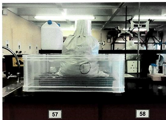
Figure 1: Example of the woven compost bags used by each group in GKD 250. The composting process was scaled down to be performed in the laboratory, yet still allows normal aerobic organic material decomposition. The woven plastic bags allow for good aeration and drainage.
