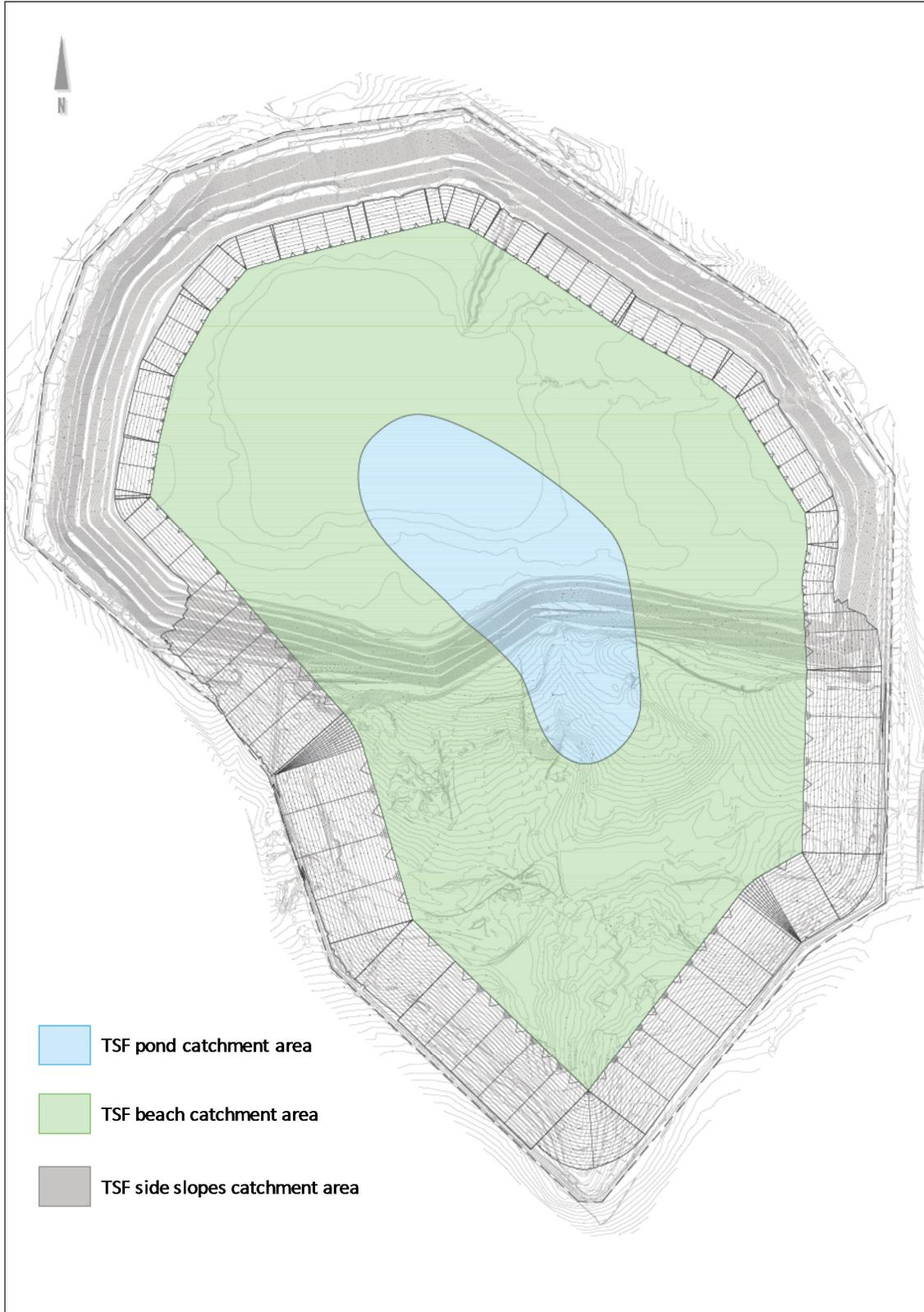
Figure 3-11: Illustration of envisaged TSF catchment area at closure
