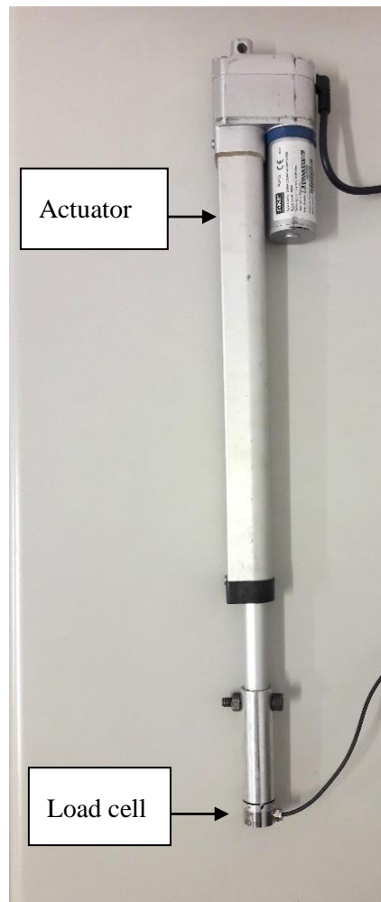
Figure 3-8. The actuator and load cell used in the experiment.
