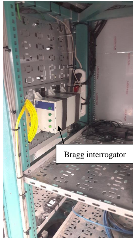
Figure 3-14. HBM fibre Bragg interrogator in the centrifuge.
