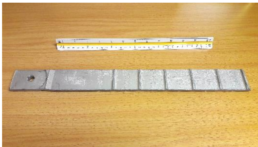
Figure 2-1. High tensile steel reinforcement strip.
