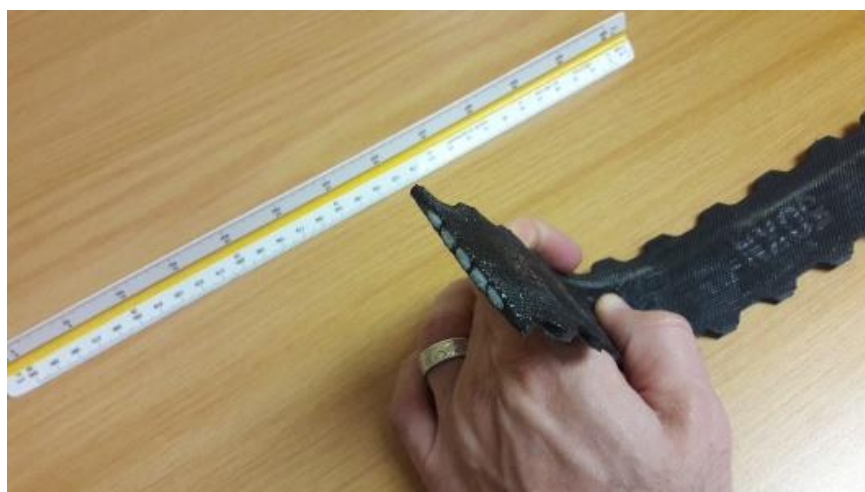
Figure 2-2. Polyester geosynthetic reinforcement strap.
