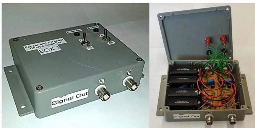
**Figure 3.50: Picture of the completed charge amplifier box**
