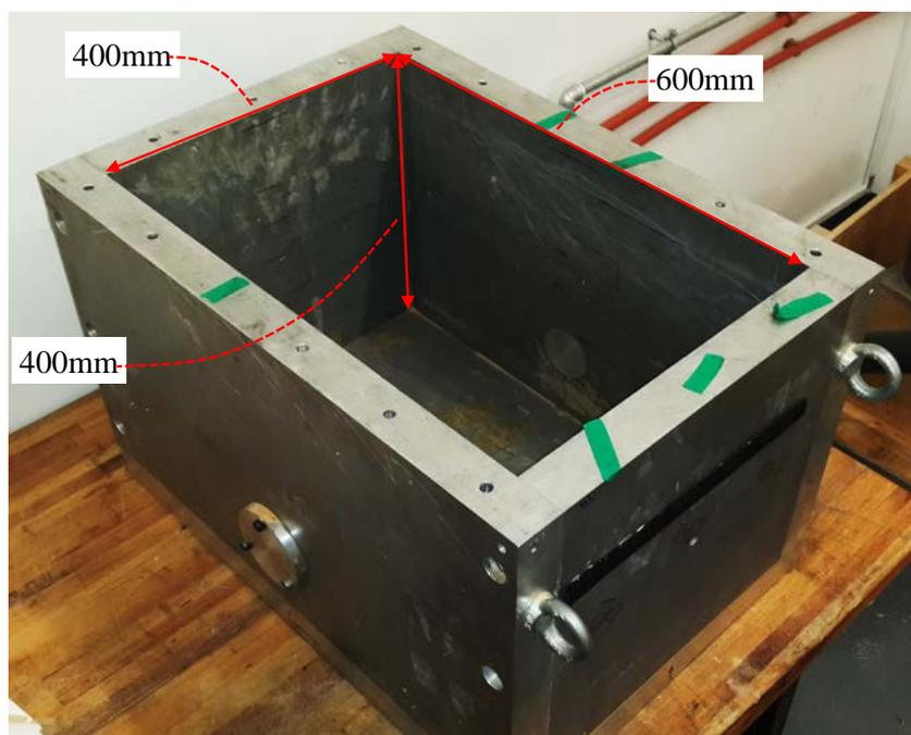
**Figure 3.40: Centrifuge model container**
