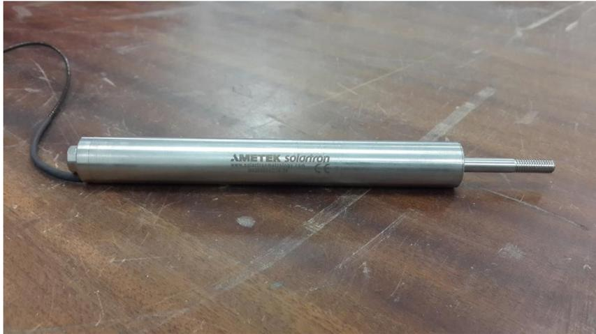
**Figure 3.60: Close-up of AS/15 S series LVDT**
