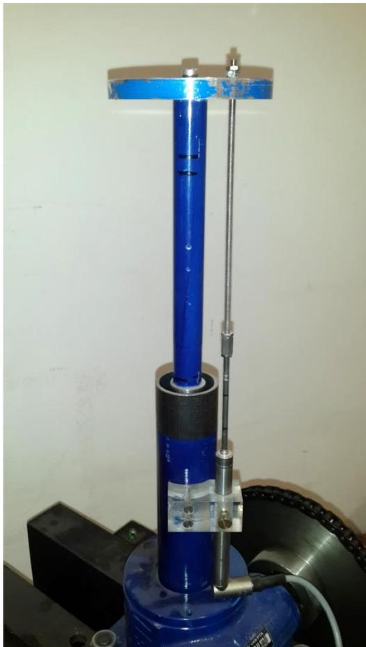
**Figure 3.57: Close up of displacement transducer attached to jack**
