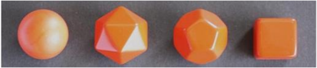
Figure 2.29: Particle shapes tested by Höhner et al. (2014) from left to right: sphere, icosahedron, dodecahedron and hexahedron
