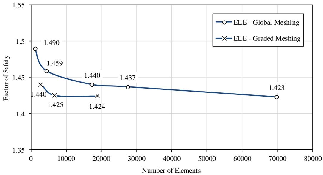
**Figure 4-12: FoS against number of elements for a global mesh size versus graded meshing**
