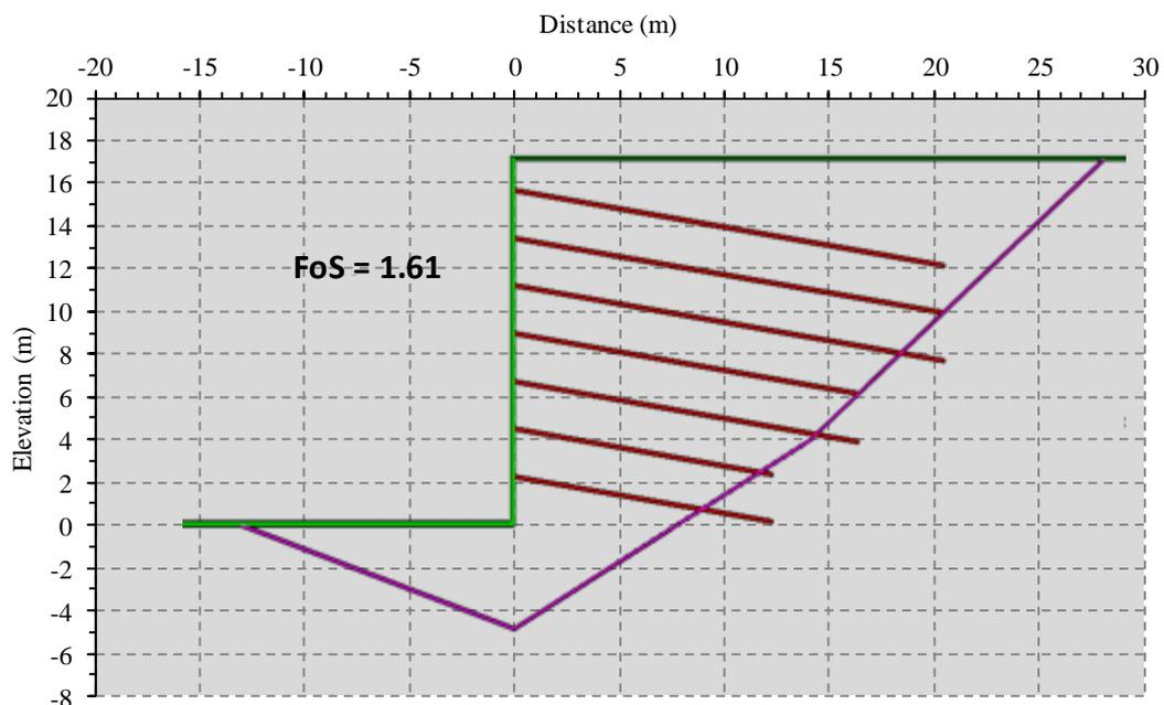
**Figure 4-77: Multiple wedge analysis for anchored excavation**
