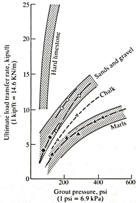
**Figure 2-13: Influence of grout injection pressure on ultimate bond capacity of anchors (Jorge, 1969)**
