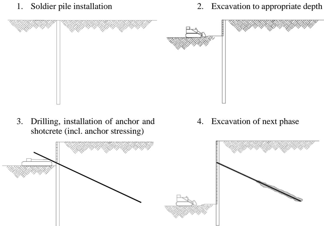
**Figure 2-15: Top-down construction sequence of anchors (FWHA, 1999)**
