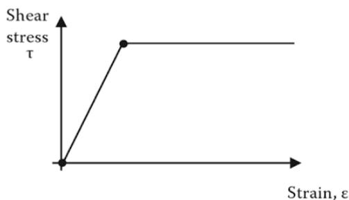
**Figure 2-24: Linear elastic perfectly-plastic (Clayton *et al.* 2013)**
