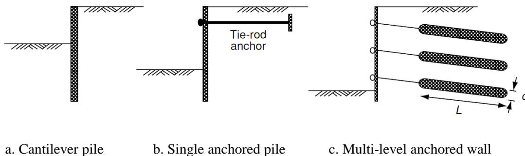
**Figure 2-16: Common embedded pile support systems (Gunaratne, 2014)**
