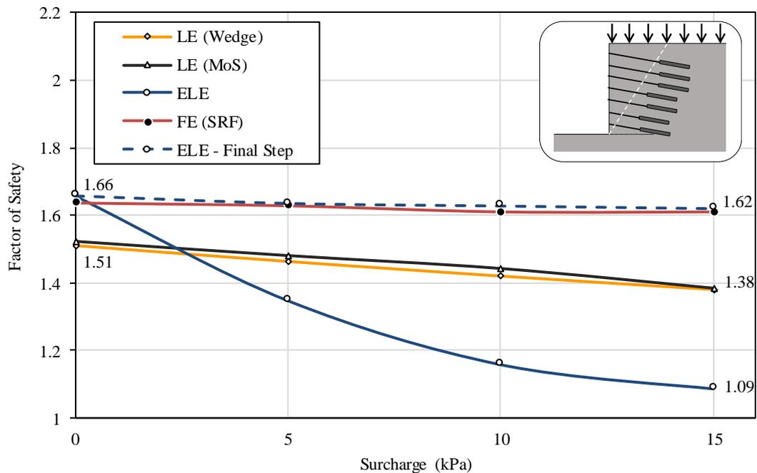
**Figure 4-63: FoS for a change surface surcharge loading**
