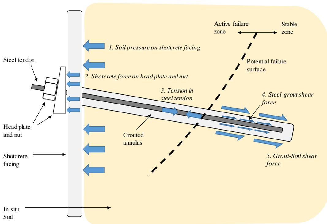
**Figure 2-4: Soil-nail system load transfer mechanism**
