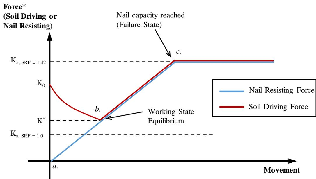
**Figure 4-34: Hypothetical loading path of soil and nails from in-situ stress to failure**
