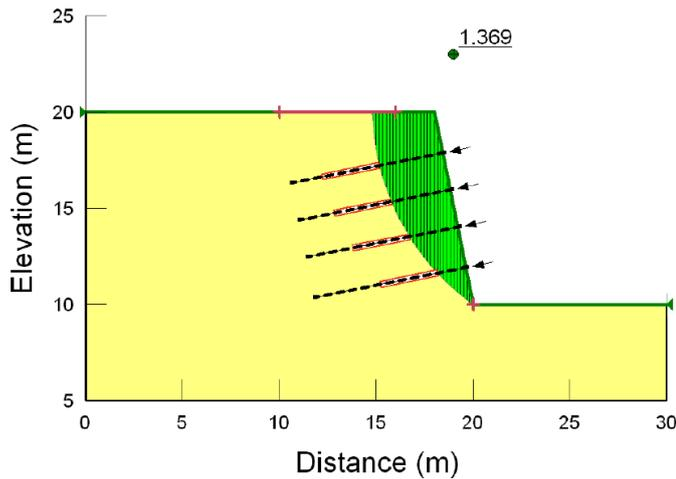
**Figure 2-32: Typical soil-nail problem analysed with Entry and Exit method**
