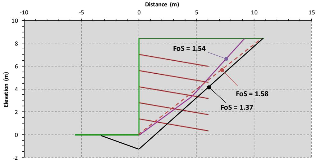
**Figure 4-75: Various failure mechanisms and FoS including planar, double and passive wedges**
