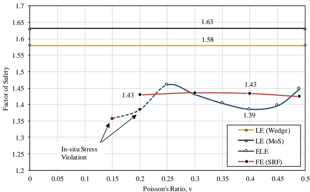
**Figure 4-22: FoS for a change in the Poisson's ratio,  $\nu'$**
