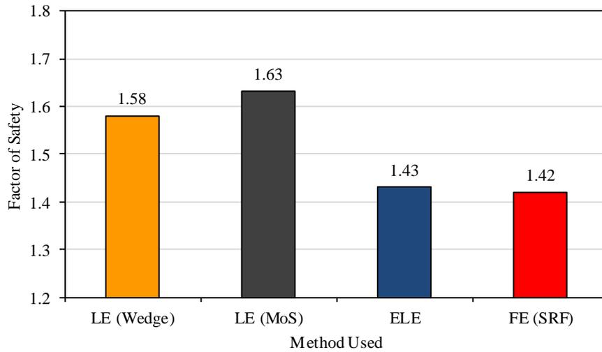
**Figure 4-8: Minimum FoS obtained from various method for soil-nailed excavation**
