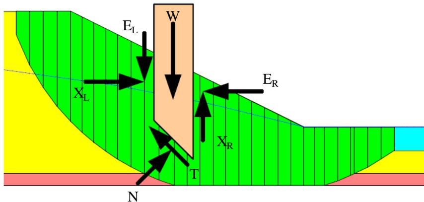
**Figure 2-27: Slice discretisation along slip surface with forces acting on a single slice (Krahn, 2003)**
