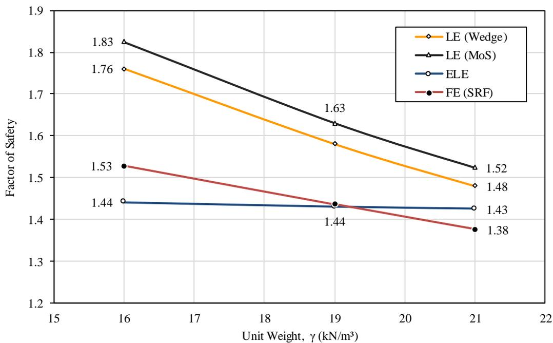
**Figure 4-20: FoS for a change in soil unit weight,  $\gamma$**
