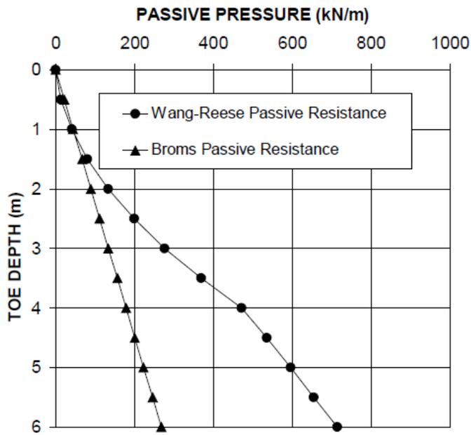
Figure 2-19: Broms and Wang-Reese comparison for lateral capacity of soldier piles (FHWA, 1999)
