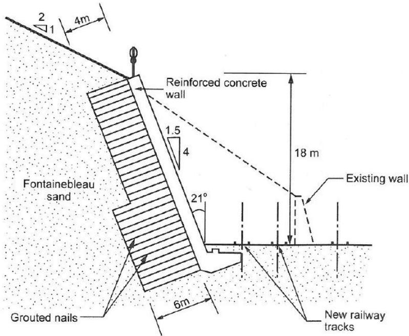
**Figure 2-2: Cross-section of soil-nail wall constructed at Versailles, France (Clouterre, 1991)**
