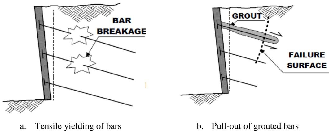
**Figure 2-6: Internal failure mechanisms (FHWA, 2003)**
