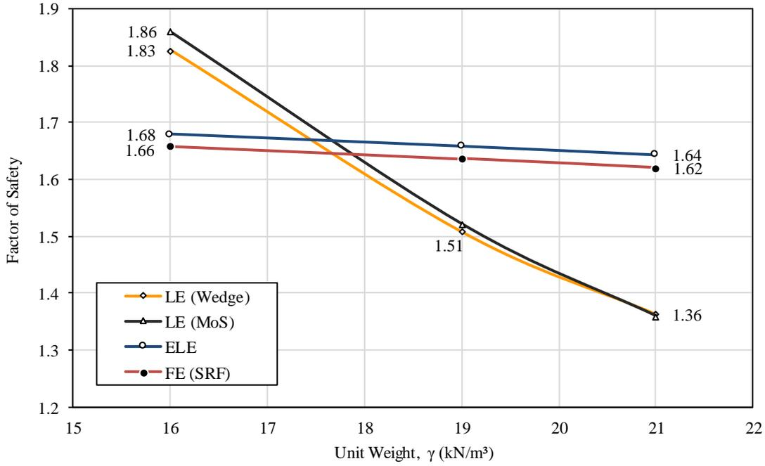
Figure 4-52: FoS for a change in unit weight,  $\gamma$
