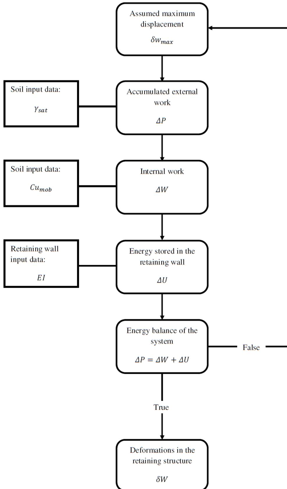
**Figure 2-39: Principle calculation procedure (Bjureland, 2013)**
