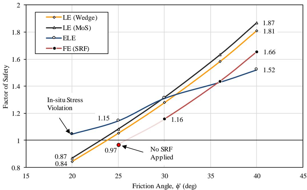
**Figure 4-18: FoS for a change in soil friction angle,  $\phi'$**
