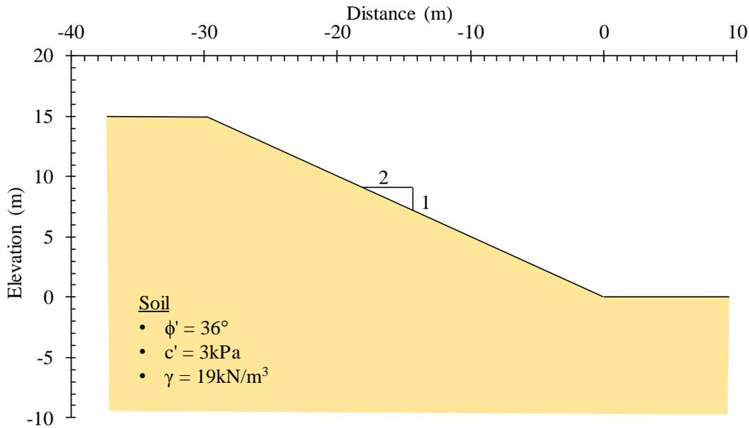
**Figure 3-1: Uniform slope cross-section**
