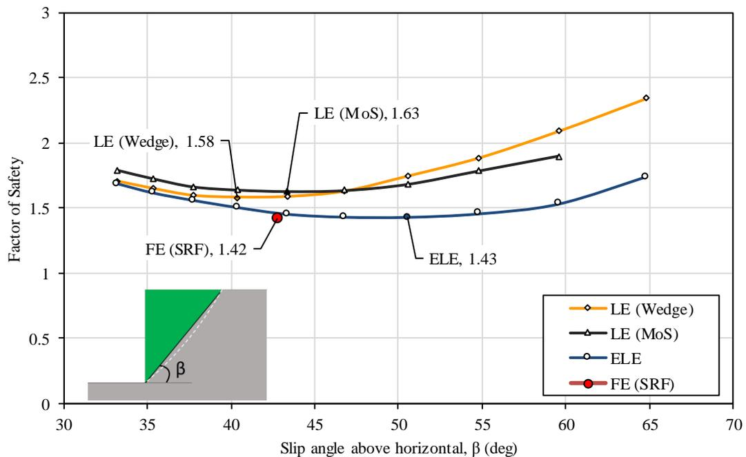
**Figure 4-7: Factor of safety for various slip angles**
