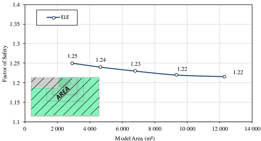
**Figure 4-42: FoS as function of the model cross-sectional area**
