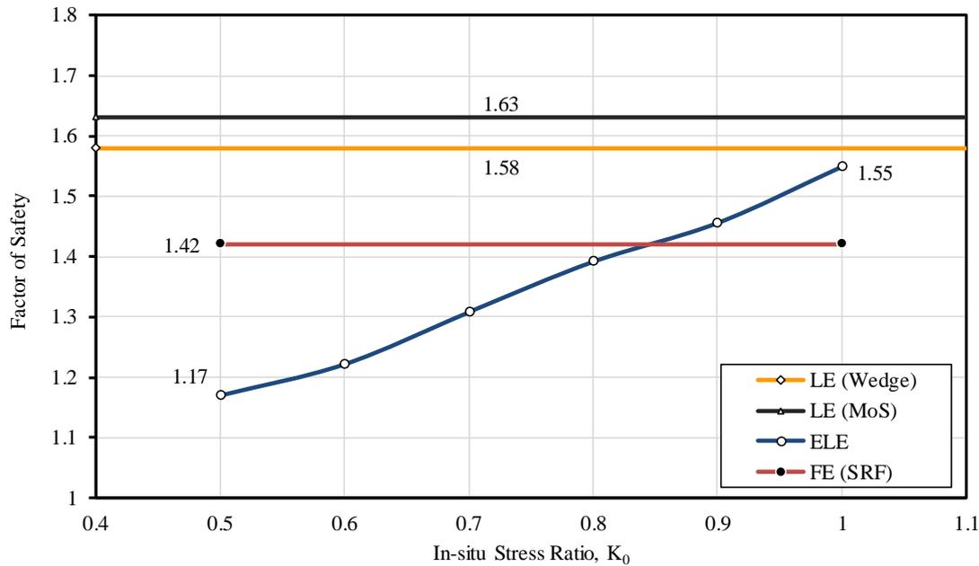
**Figure 4-33: FoS for a change in In-situ Stress Ratio,  $K_0$**
