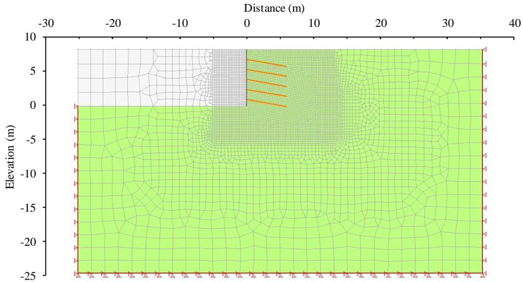
**Figure 4-11: Graded meshing model for ELE Method**
