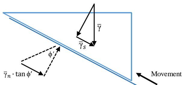
**Figure 4-51: Force diagram along passive wedge rupture surface**
