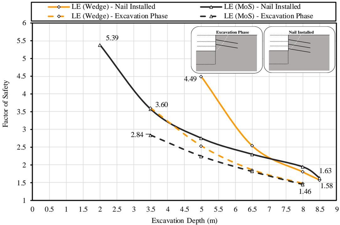
Figure 4-28: FoS against excavation depth for Wedge Method and MoS
