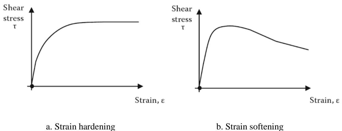
**Figure 2-23: Strain hardening or softening materials (Clayton *et al.* 2013)**
