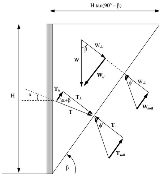
**Figure 2-42: Forces considered on a trial wedge**
