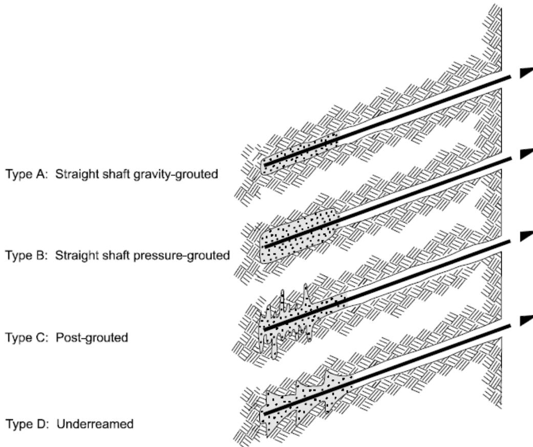
**Figure 2-11: Main types of grouted ground anchors (Littlejohn, 1990)**
