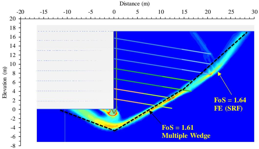
**Figure 4-78: Comparable failure mechanisms for FE (SRF) Method and multiple wedge analysis using anchor yield capacity**
