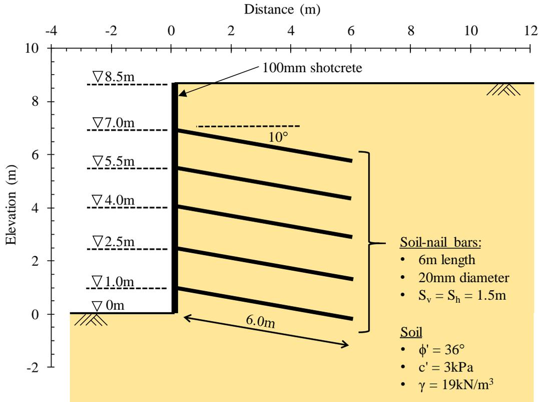
**Figure 4-6: Cross-section A-A showing soil-nailed details**
