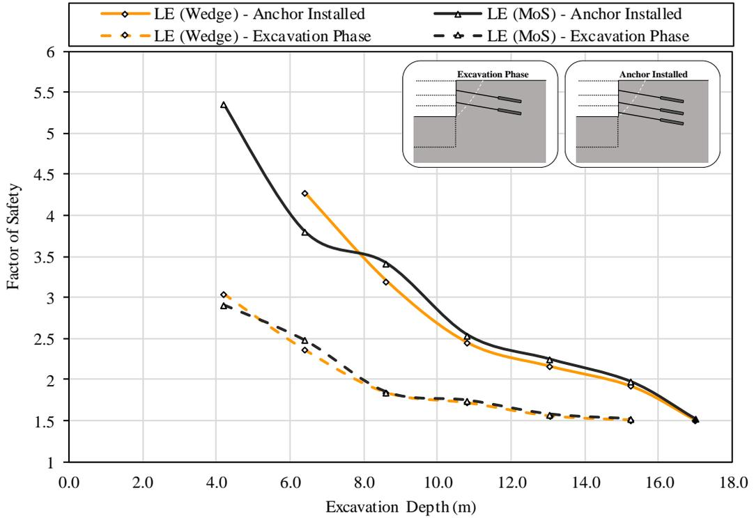
Figure 4-64: FoS against excavation depth for Wedge Method and MoS
