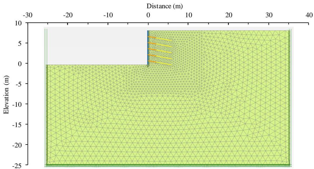
**Figure 4-17: FE (SRF) graded mesh model with 2 010m<sup>2</sup> cross-sectional area and 5 198 elements**
