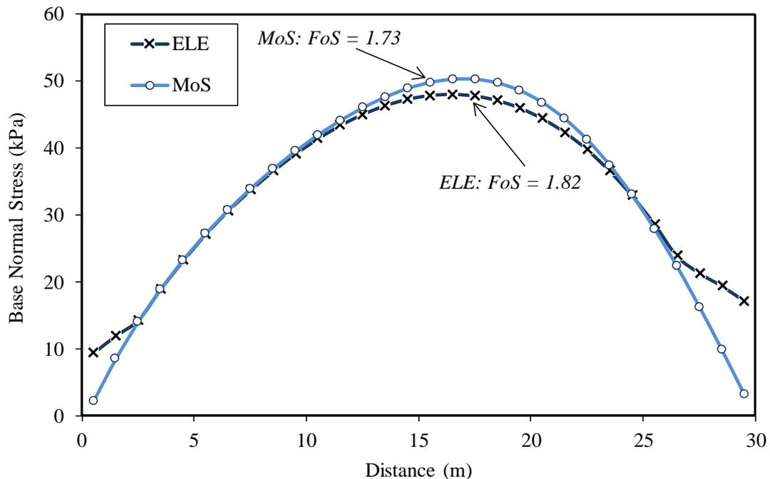
**Figure 4-3: Normal stress distribution along slip surface**
