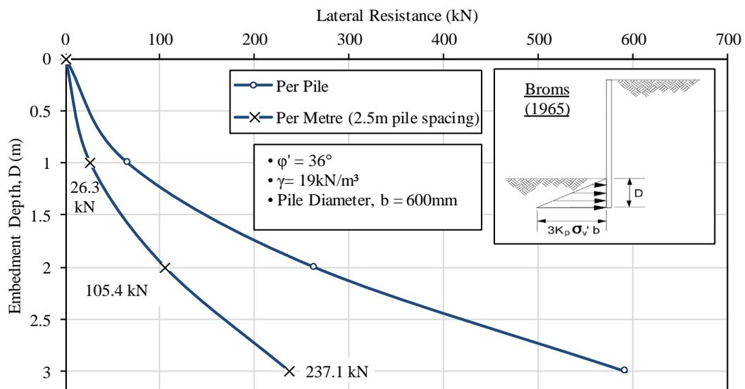
**Figure 4-67: The lateral resistance of piles as a function of embedment depth according to Broms (1965)**
