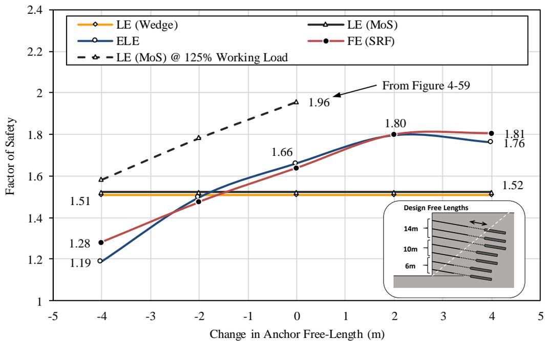
**Figure 4-61: FoS for a change in anchor free-length**
