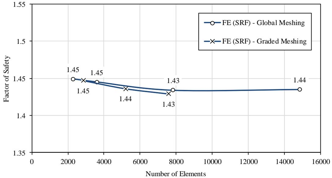
**Figure 4-15: FoS against number of elements for a global mesh size versus graded meshing for FE (SRF) model**
