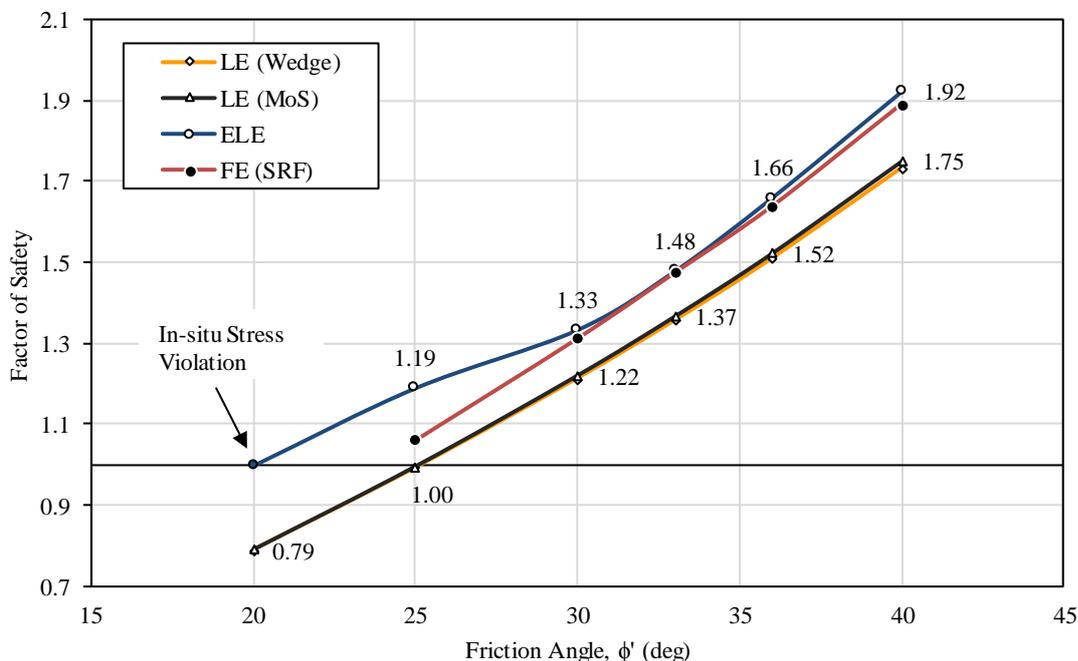
**Figure 4-47: FoS for a change in friction angle,  $\phi'$**
