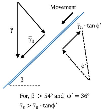
**Figure 4-50: Force diagram along an inclined rupture surface**
