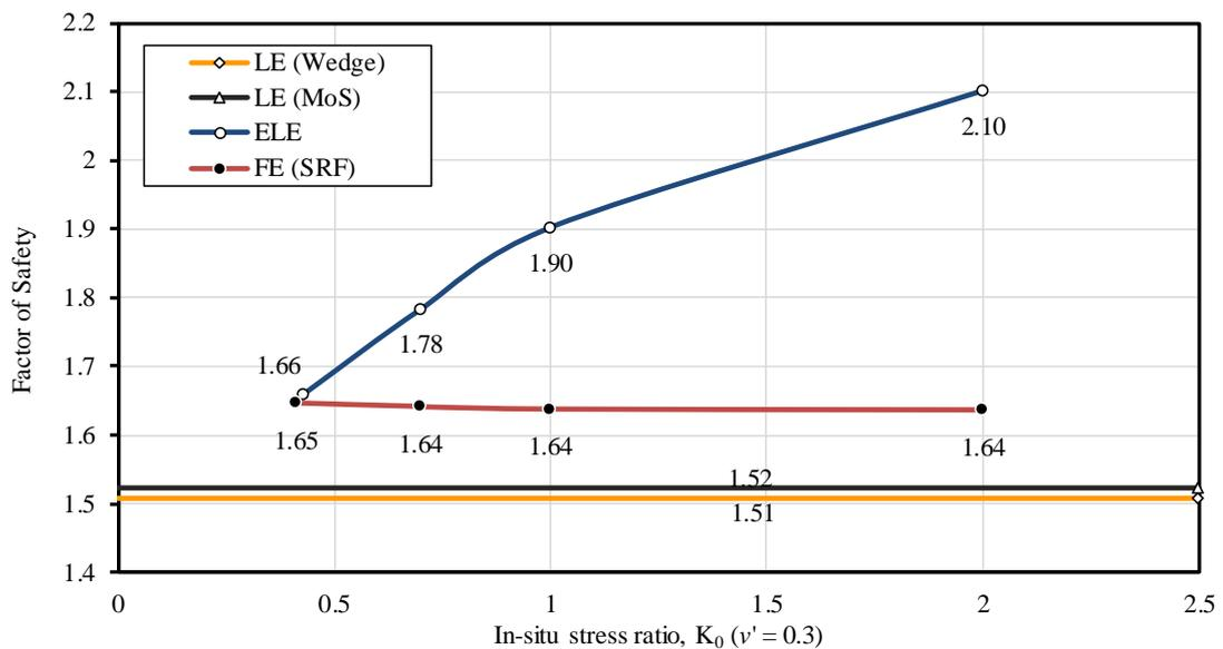
**Figure 4-57: FoS for a change in in-situ stress ratio,  $K_0$  ( $v' = 0.3$ )**
