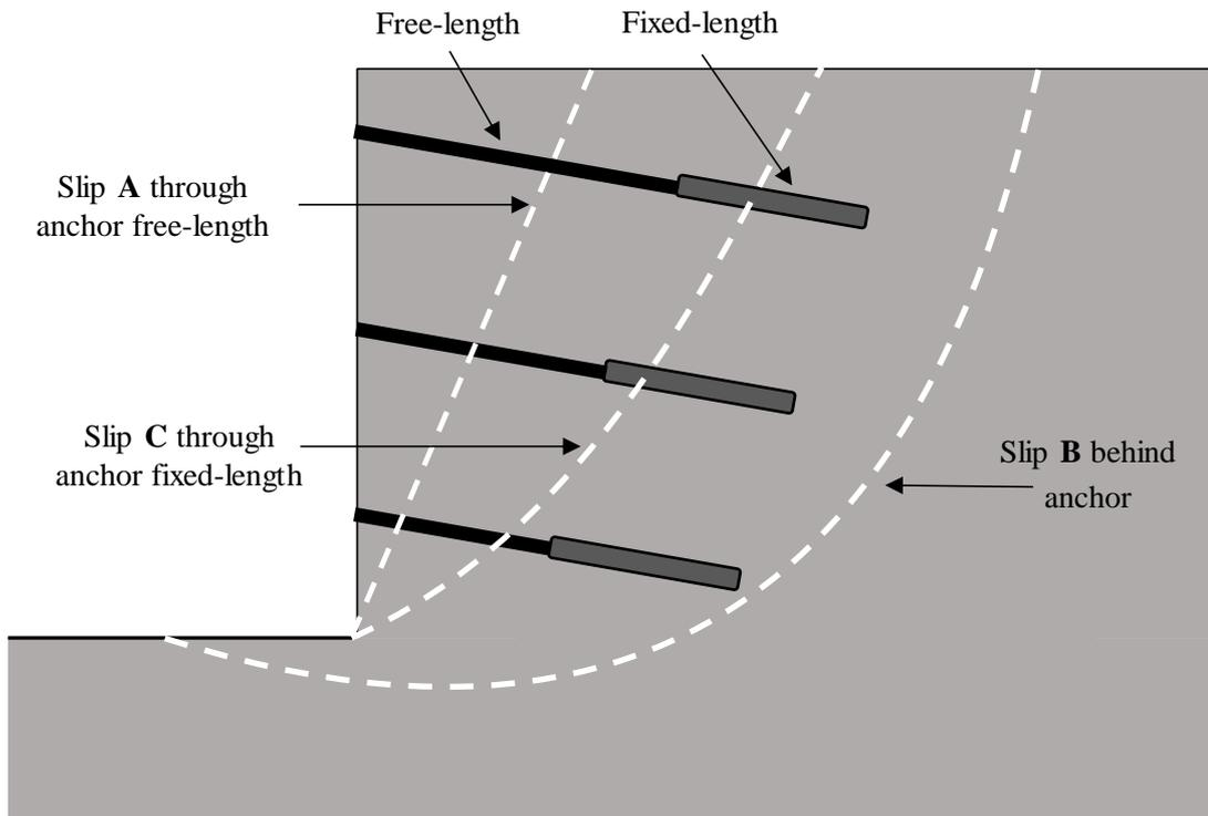
**Figure 3-4: Possible slip surfaces for anchors**
