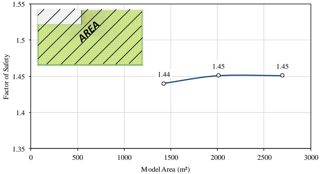
**Figure 4-16: FoS against number of elements for a global mesh size**
