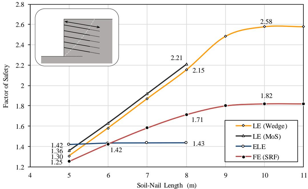
**Figure 4-25: FoS for a change nail design length**
