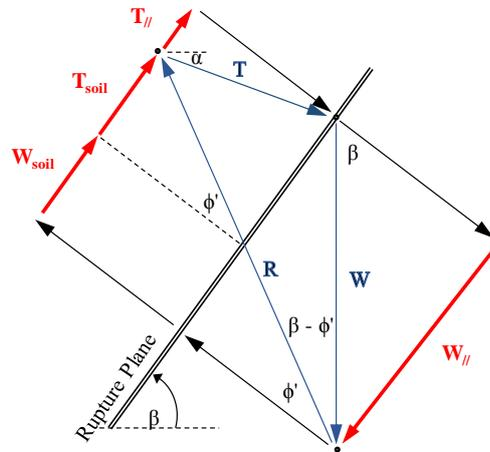
**Figure 2-43: Force polygon with parallel and perpendicular components to the rupture plane**
