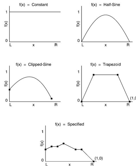
**Figure 2-29: Typical interslice force functions for Morgenstern-Price Method (SLOPE/W 2012)**
