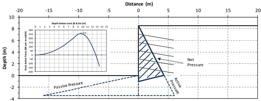
**Figure 4-76: Rankine's active, passive and net pressure diagrams for soil-nailed excavation**
