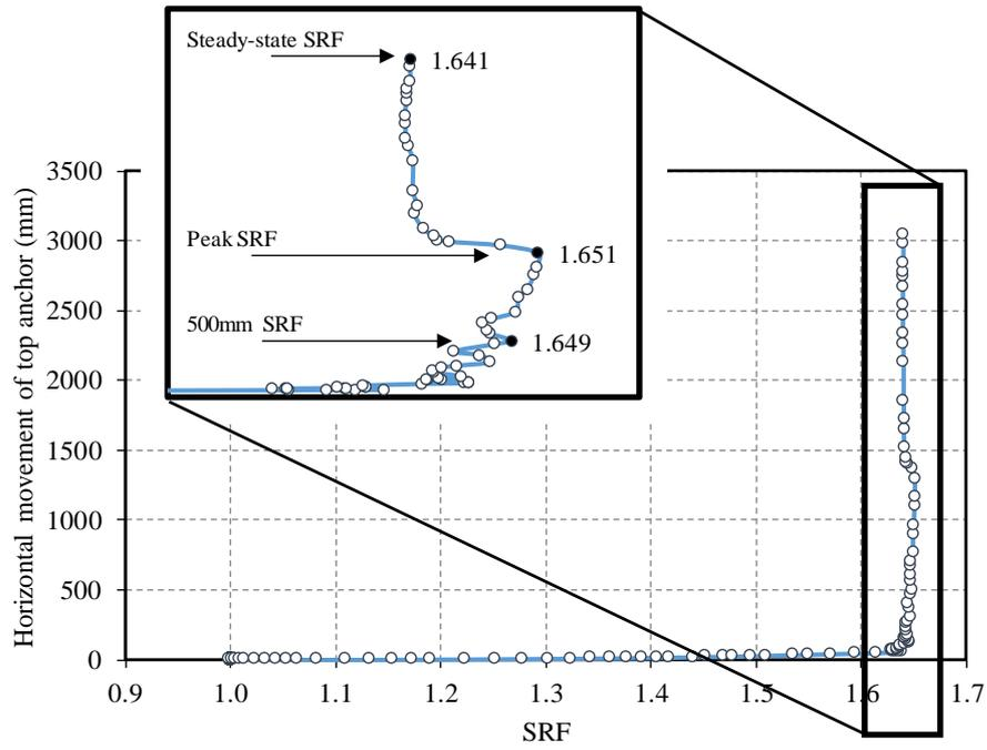
**Figure 3-7: Strength Reduction Factor against horizontal movement of the top anchor head**
