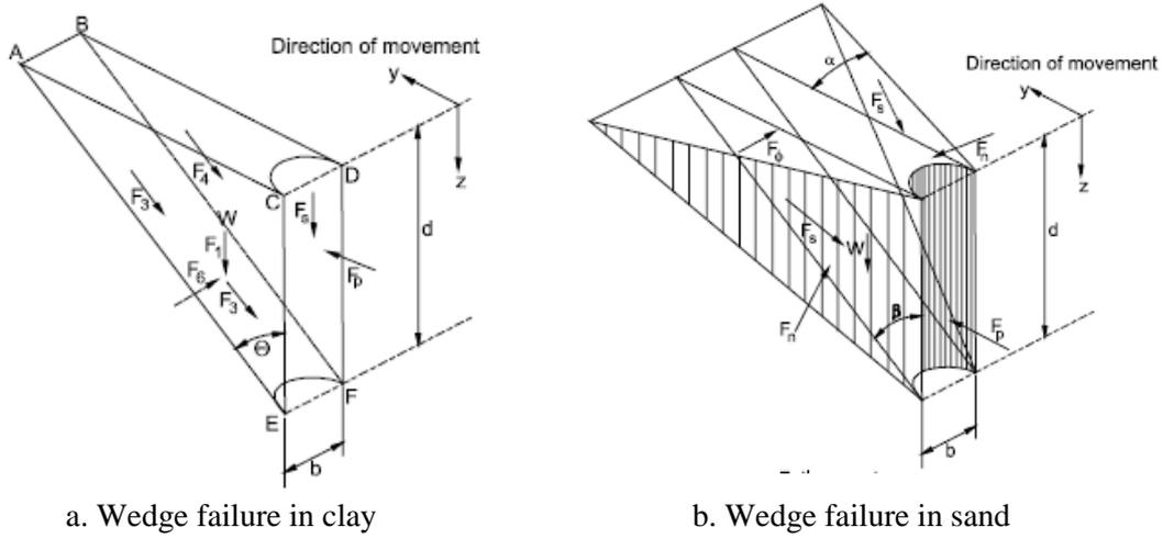
Figure 2-18: Wang-Reese failure wedge in sands and clays (FHWA, 1999)
