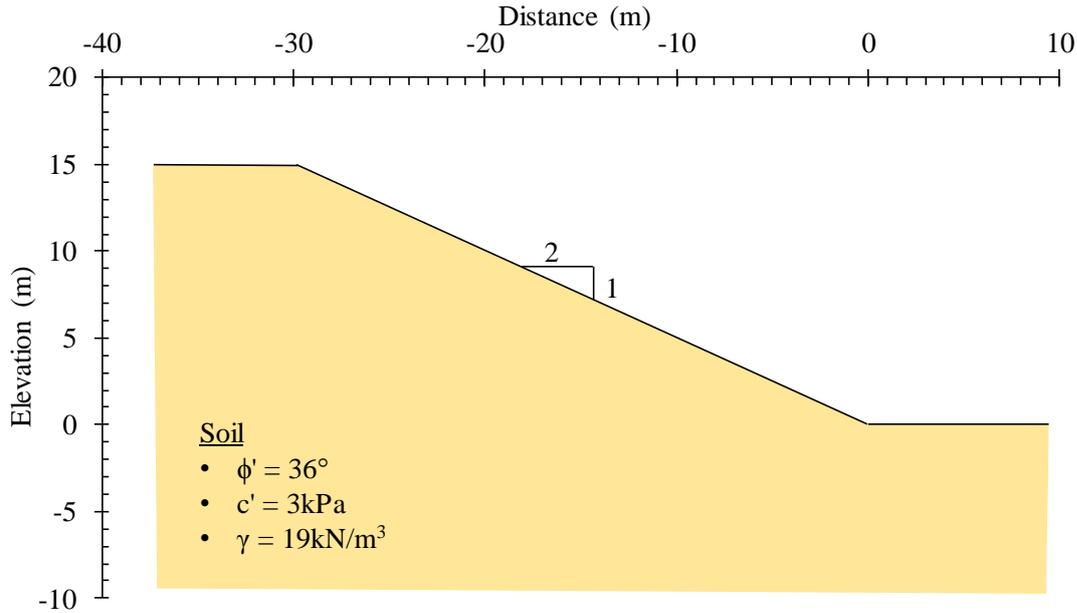
**Figure 4-1: Uniform slope cross-section**
