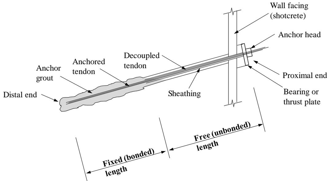
Figure 2-9: Anchor basic components (after SAICE, 1989)
