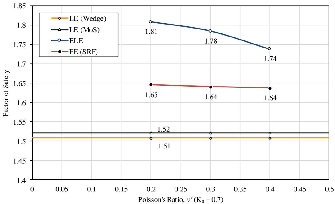
**Figure 4-56: FoS for a change in Poisson's Ratio,  $\nu'$  ( $K_0 = 0.7$ )**
