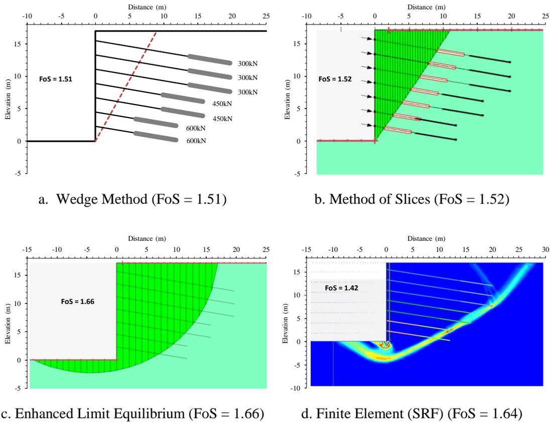
Figure 4-40: Anchored excavation critical failure mechanisms and associated factors of safety
