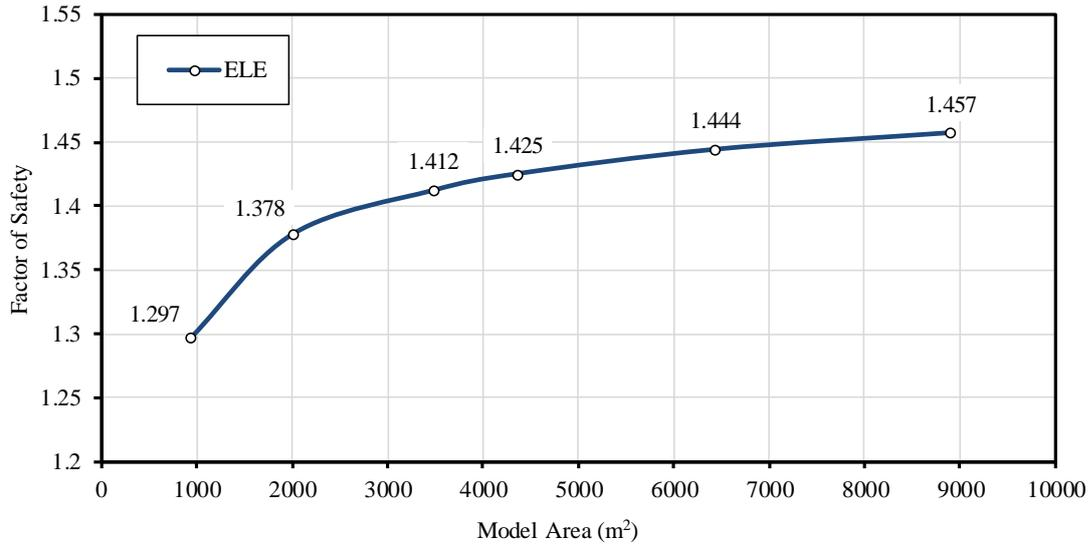
**Figure 4-14: FoS as function of the model cross-sectional area**
