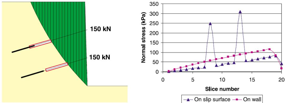
**Figure 2-33: Normal stress distribution along slip surface for anchored lateral support (Krahn, 2003)**
