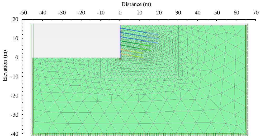
**Figure 4-46: FE (SRF) graded mesh model with 6 270m<sup>2</sup> cross-sectional area and 2 556 elements**
