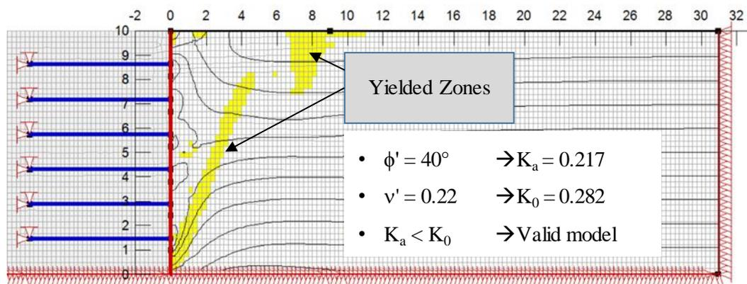
**Figure 4-70: Cross-section propped excavation showing valid in-situ stresses**
