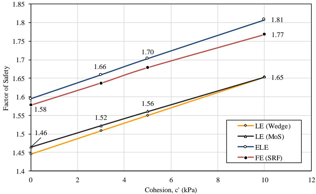
**Figure 4-49: FoS for a change in cohesion,  $c'$**
