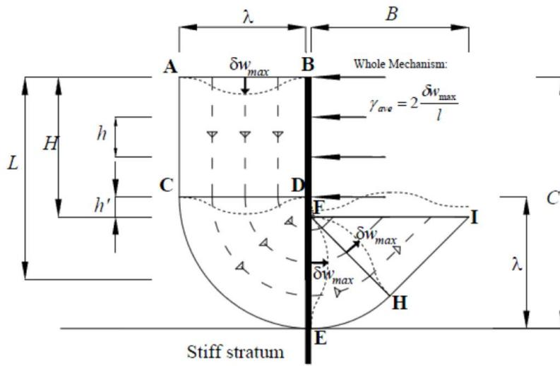
Figure 2-40: Displacement field for braced excavation (Osman & Bolton, 2006)
