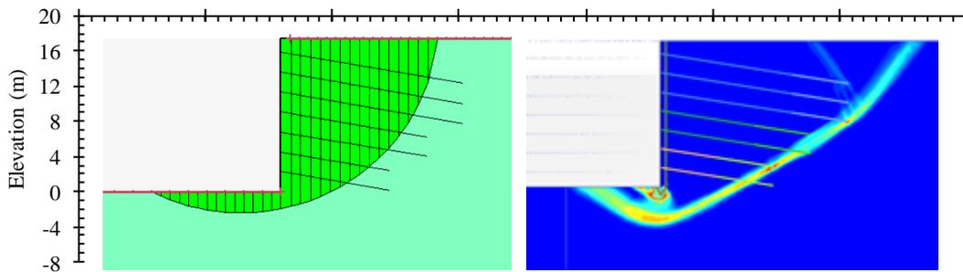
Figure 4-54: Deep failure surface inclinations (left - ELE Method ; right - FE (SRF) Method)
