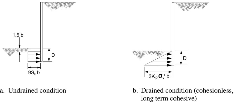
**Figure 2-17: Broms method for evaluating the ultimate lateral capacity of embedded piles (FHWA, 1999)**
