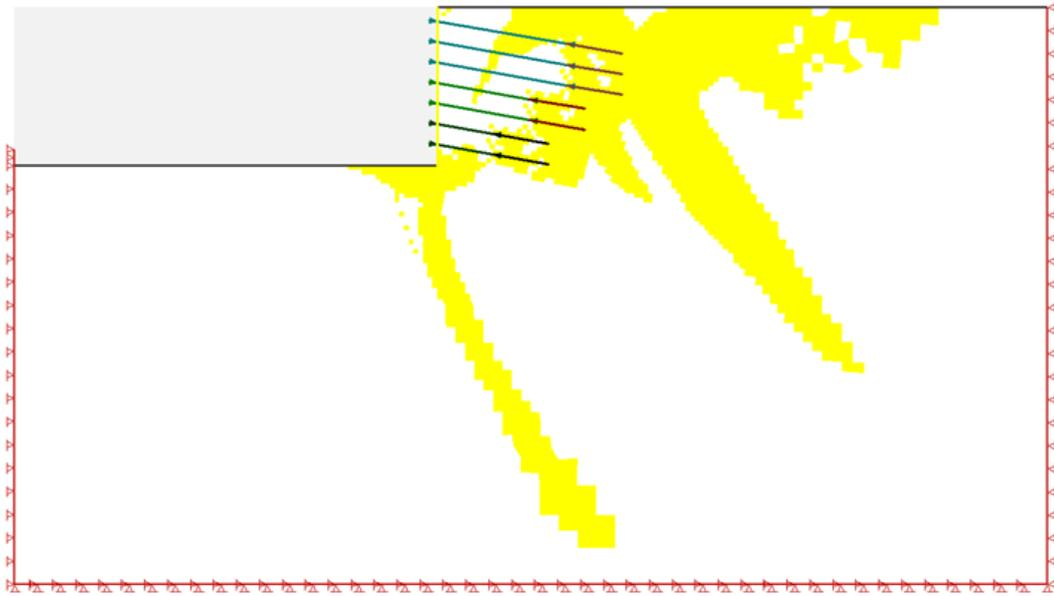
**Figure 4-48: ELE Method yielding zones for friction angle,  $\phi' = 25^\circ$  and  $\nu' = 0.3$**
