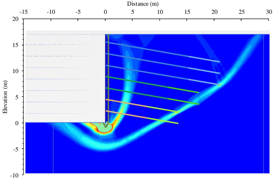
**Figure 4-62: Shadings of incremental shear strain for free-lengths increased by 2m**
