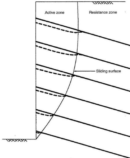
**Figure 2-5: Nail deformation mechanism (Mitchell and Villet, 1987)**
