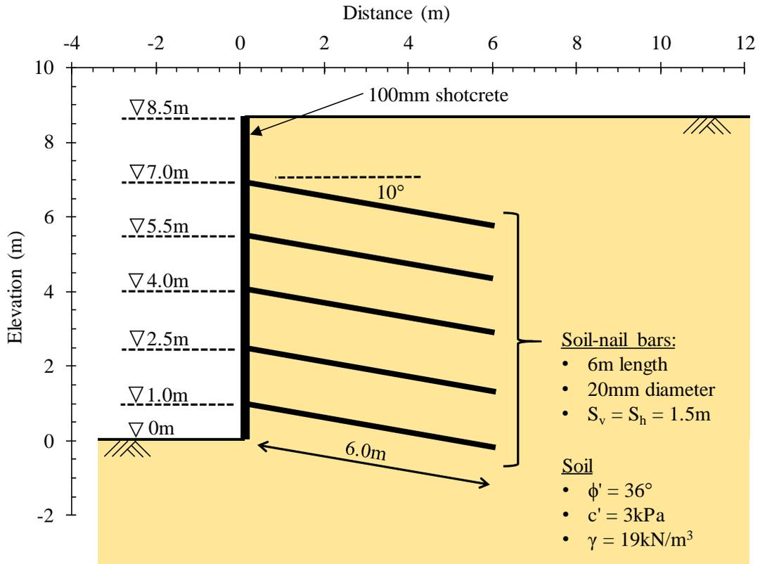
**Figure 3-2: Soil-nailed excavation design**
