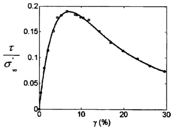
Figure 2-41: Stress-strain response of Norwegian quick clay (Bjerrum & Landva, 1966)
