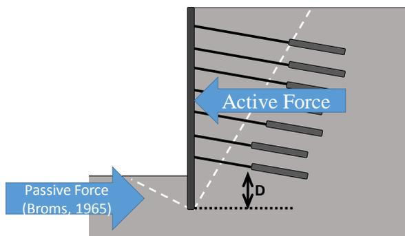
**Figure 4-66: Broms' theory applied to Wedge Method and MoS**
