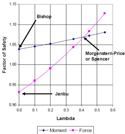
**Figure 2-28: Factor of Safety versus Lambda,  $\lambda$ , plot (SLOPE/W, 2012)**
