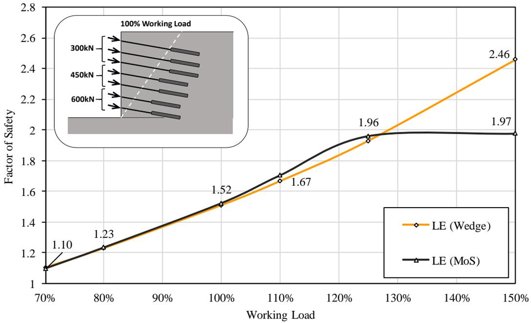
**Figure 4-59: FoS for a change in anchor working load for the Wedge Method and MoS**
