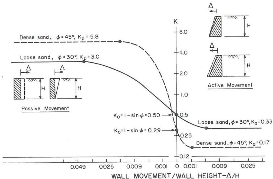
**Figure 2-20: Relationship between wall movement and earth pressure for ideal cases of walls “wished into place” (Fang, 1991).**
