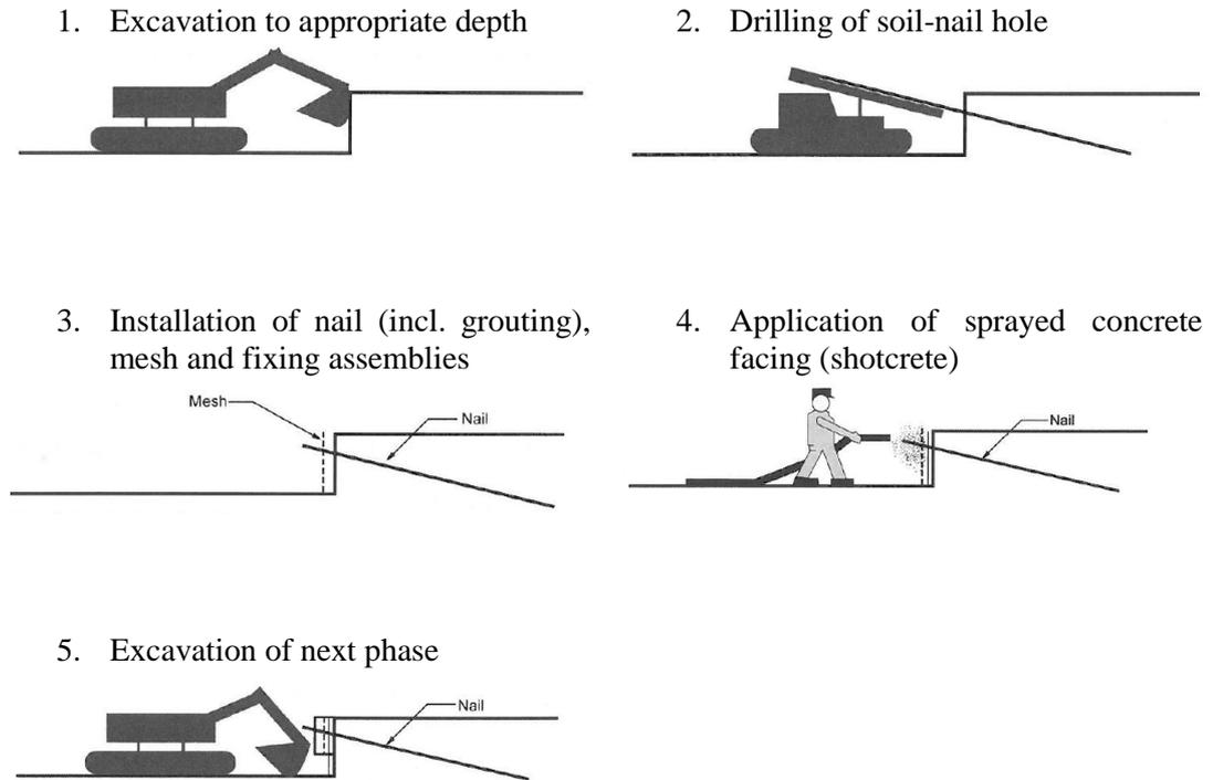
**Figure 2-8: Top-down construction sequence of soil-nails (CIRIA, 2005)**
