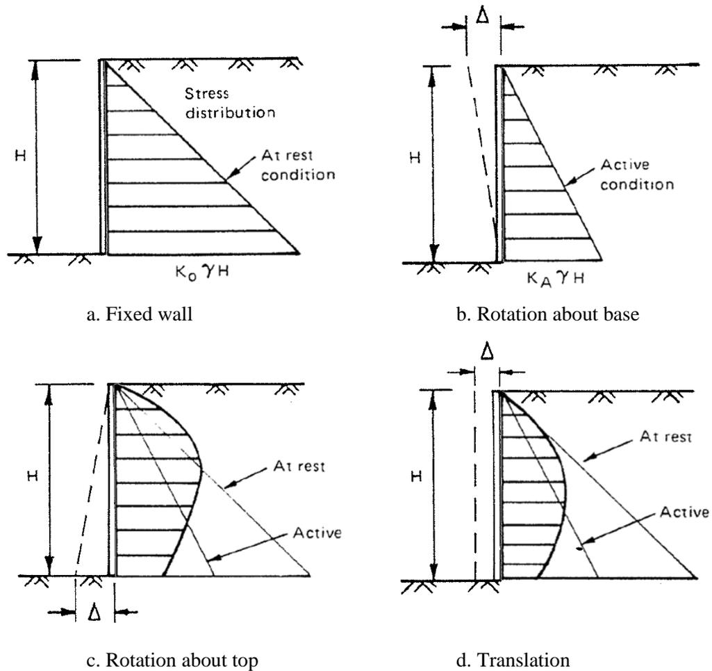
**Figure 2-21: Reduction in earth pressure due to movement mechanism (Mc Gown *et al.* 1987)**
