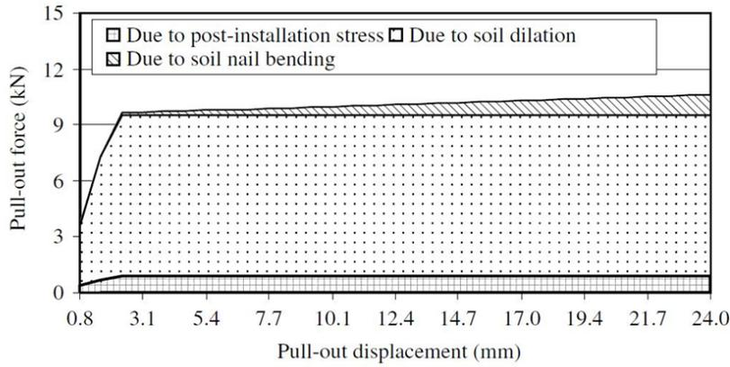
**Figure 2-7: Pull-out resistance contributions due to vertical pressure, dilatancy and bending (Zhou & Yin, 2008)**
