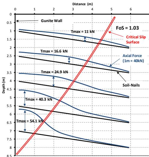
c. Full stage construction model with specified in-situ stresses
