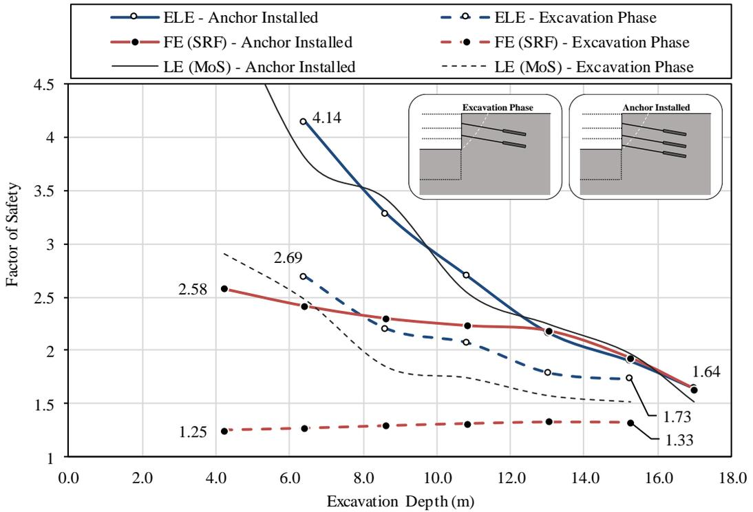
Figure 4-65: FoS against excavation depth for ELE and FE (SRF) Methods
