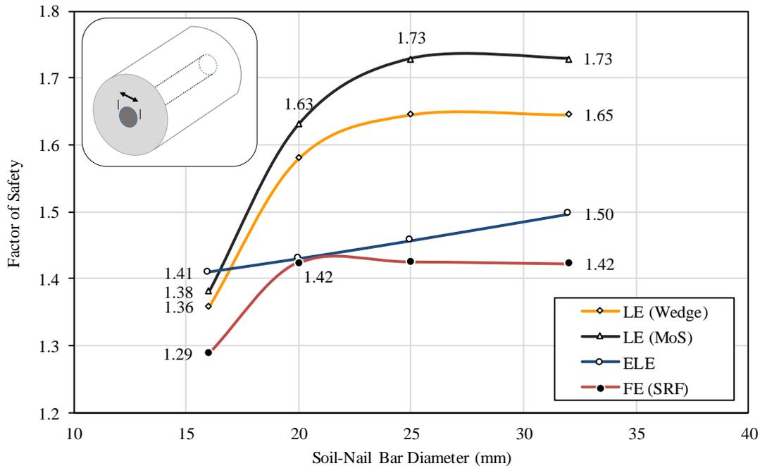
**Figure 4-24: FoS for a change in nail diameter.**
