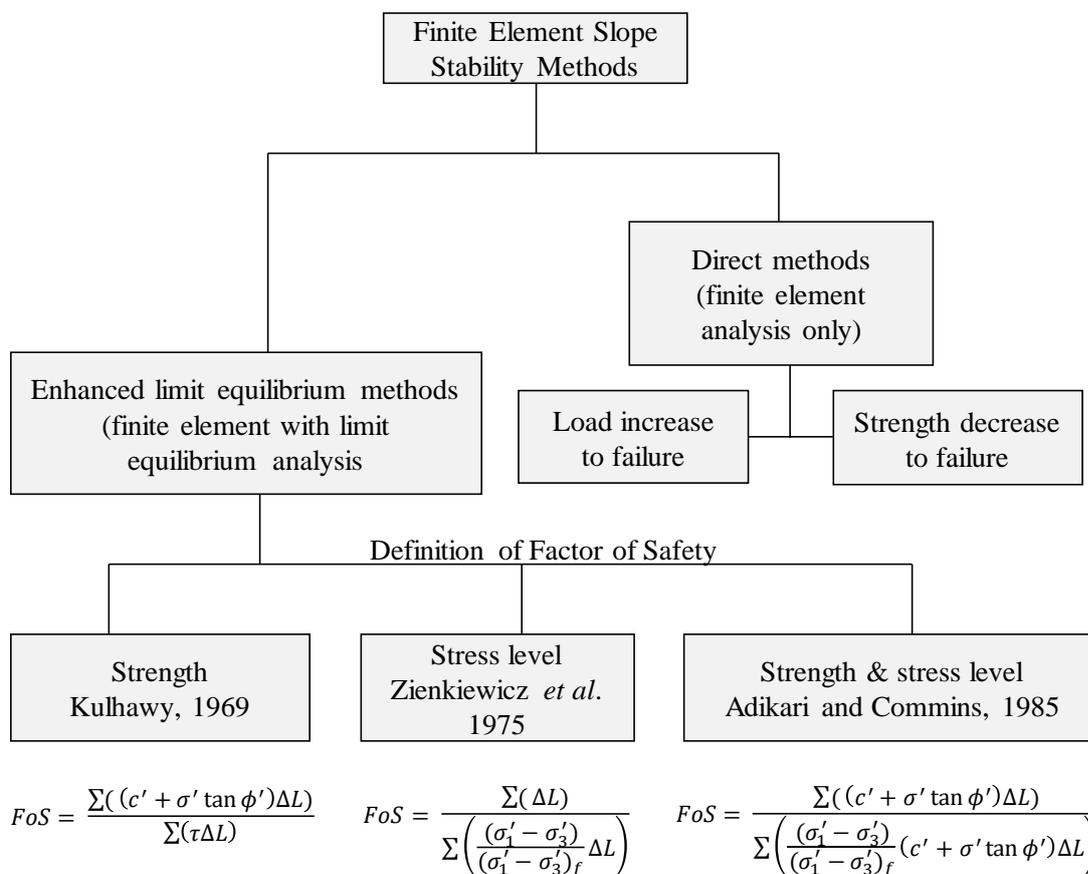
**Figure 2-34: Flow chart of finite element slope stability methods (Fredlund & Scoular, 1999)**
