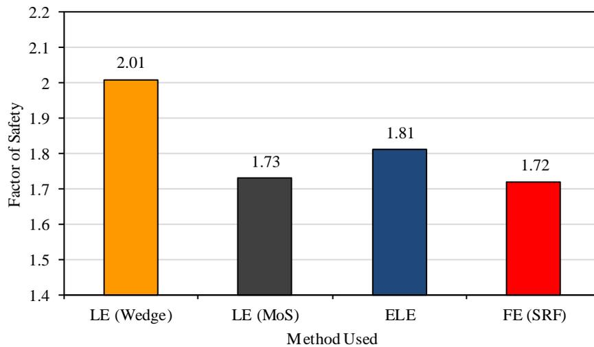
**Figure 4-4: Minimum FoS obtained from various methods for uniform slope**
