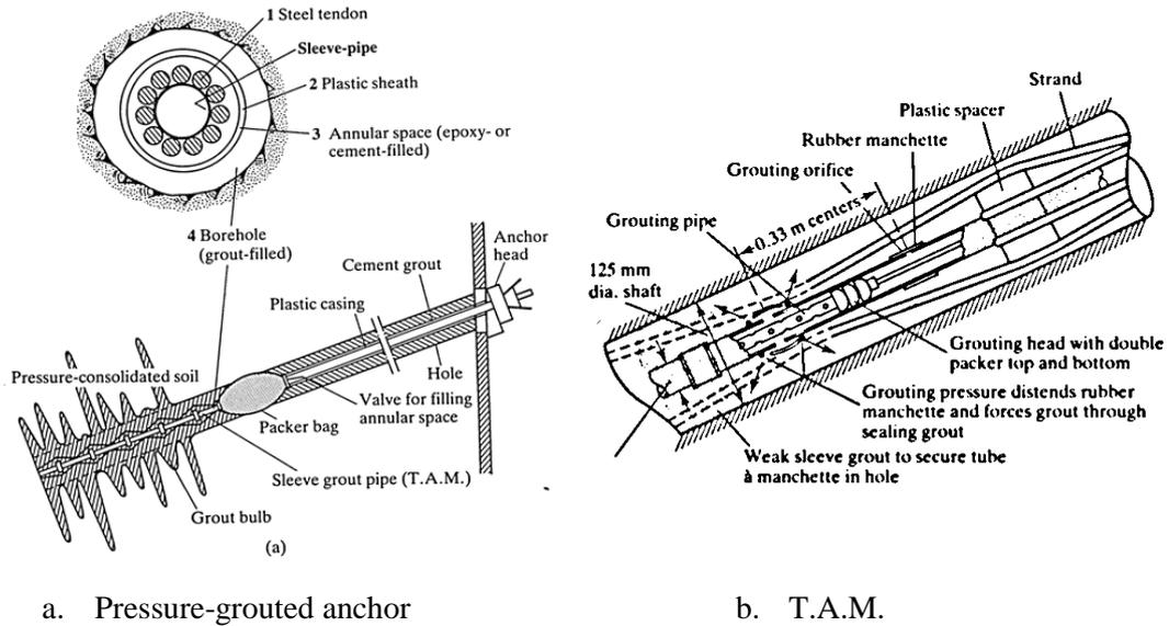
**Figure 2-12: High pressure post-grouted anchors using a T.A.M system. Example of Soletanche IRP anchor (Pfister *et al.* 1982)**
