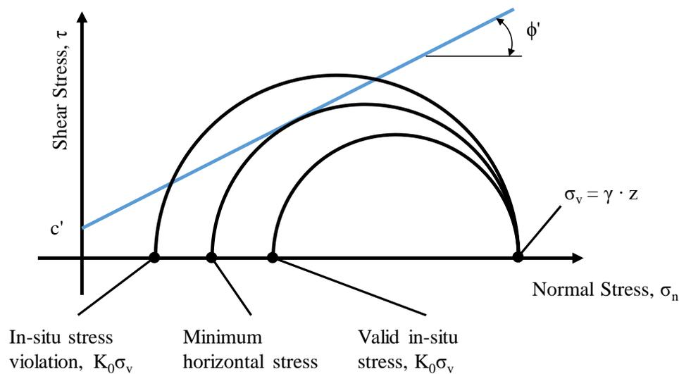
**Figure 4-69: Mohr-circle of stress showing valid, invalid and minimum stress conditions**
