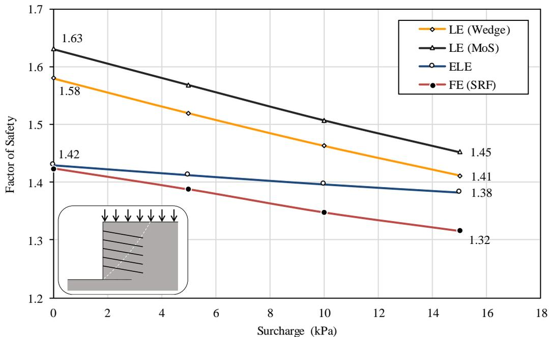
**Figure 4-26: FoS for a change in surface surcharge**
