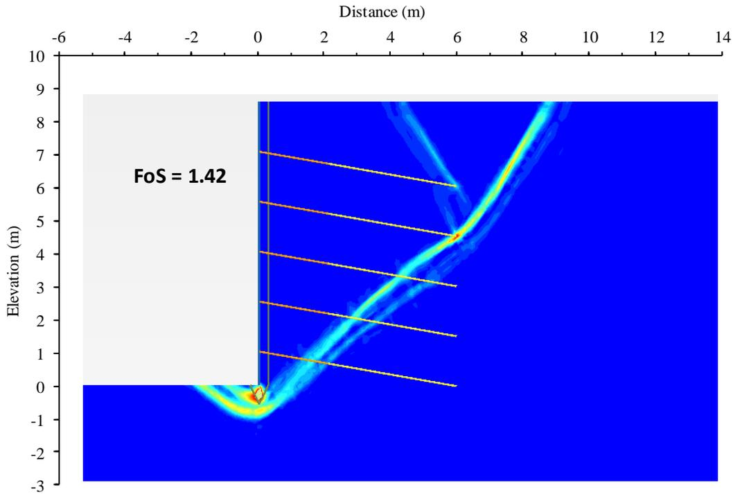
**Figure 4-73: FE (SRF) Method showing shadings of incremental shear strain at failure for soil-nailed excavation**
