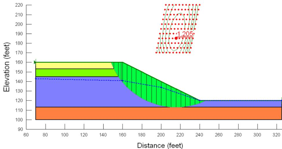
**Figure 2-31: Typical slope stability problem using grid and radius search method**
