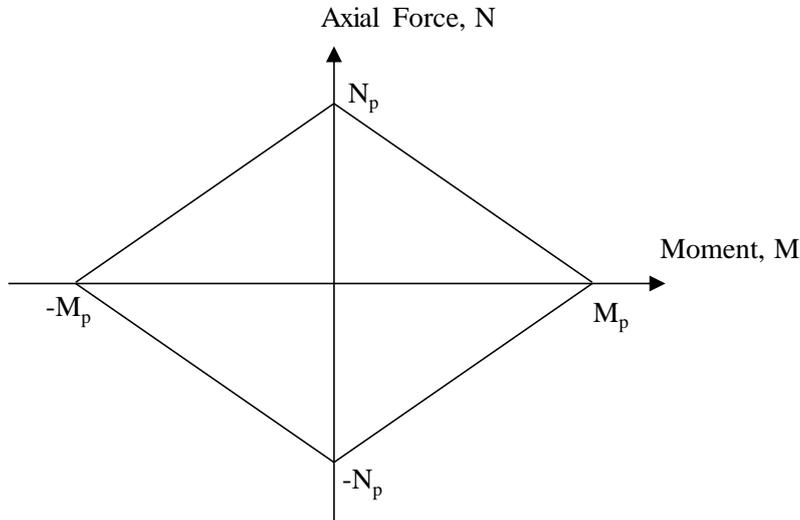
**Figure 2-38: Maximum/plastic force-moment loading combination (PLAXIS, 2016)**
