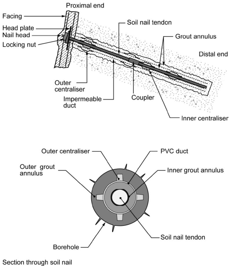
**Figure 2-3: Soil-nail main components (CIRIA, 2005)**
