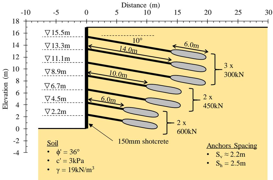
Figure 3-3 shows a cross-section of the anchored excavation design layout and basic parameters.
