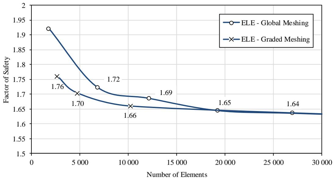
**Figure 4-41: FoS against number of elements for a global mesh size and graded meshing**
