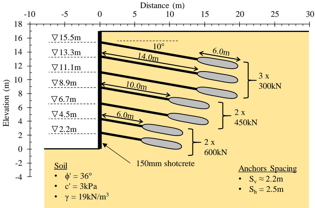
**Figure 4-37: Cross-section showing anchor details**
