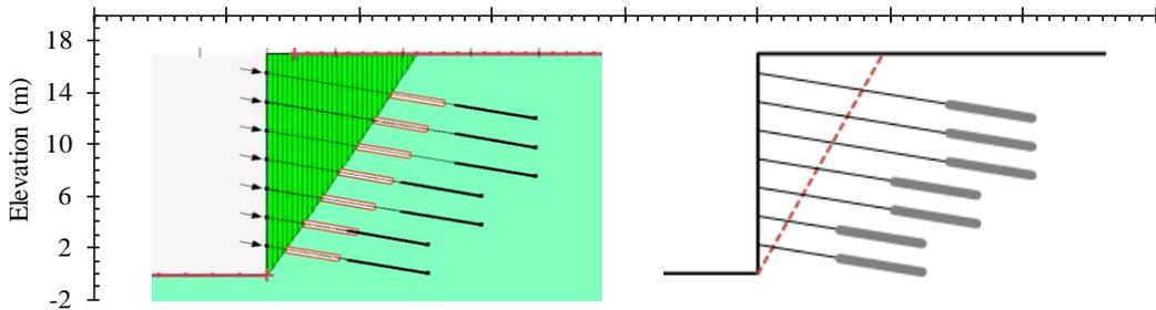
Figure 4-53: Steep failure surface inclinations (left - Wedge Method ; right - MoS)
