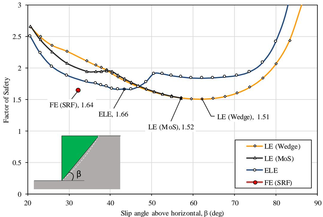
**Figure 4-38: Factor of safety for various slip angles**
