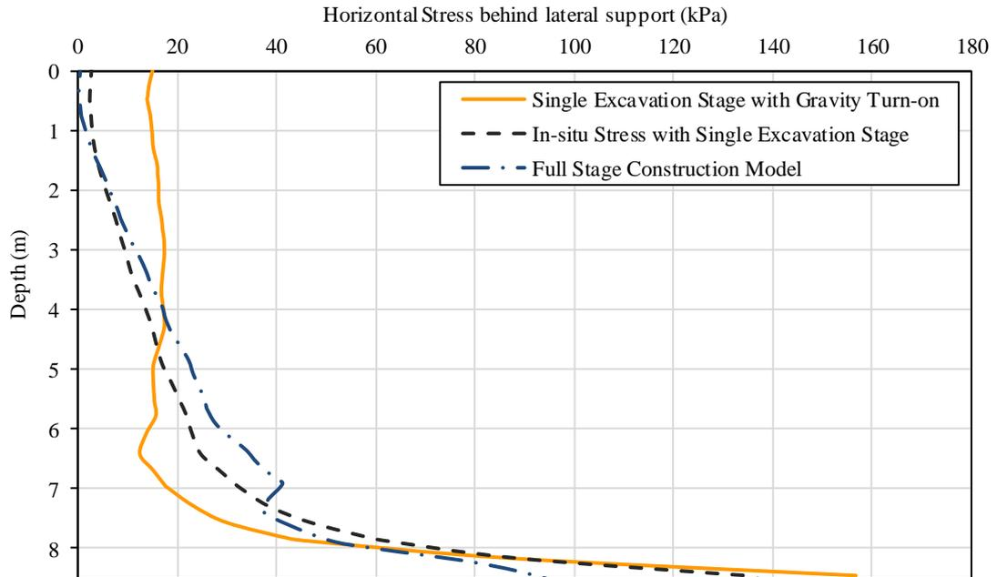
**Figure 4-30: Horizontal pressure behind retained face for three different analysis procedures using ELE Method**
