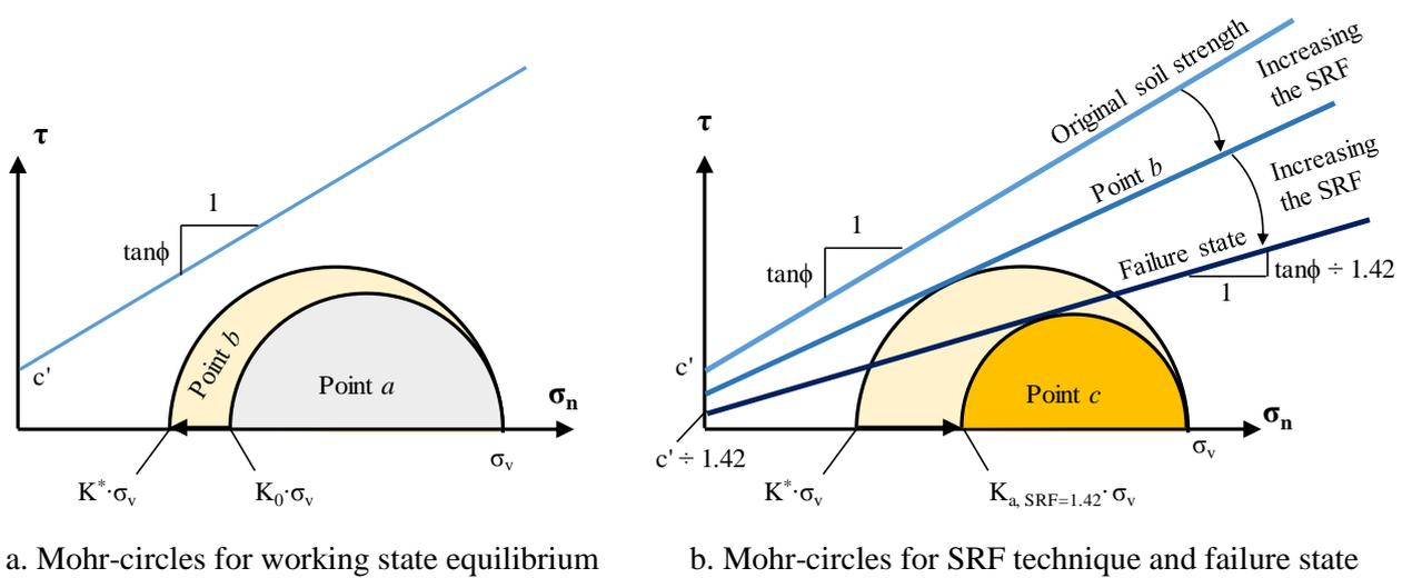
**Figure 4-35: Mohr-circles of stress for hypothetical loading path**
