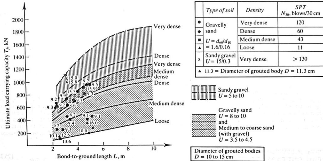
**Figure 2-14: Ultimate load holding capacity of anchors in cohesionless soils (After Ostermayer and Scheele, 1977)**
