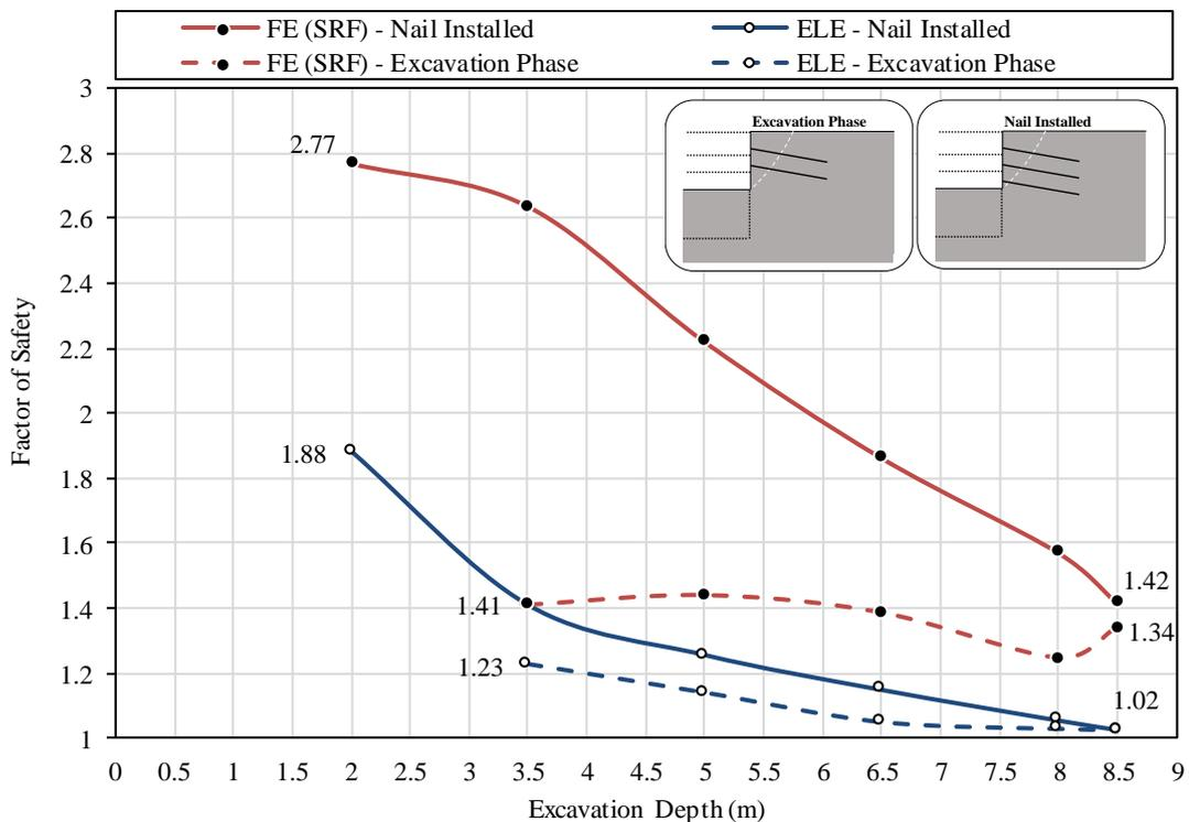
**Figure 4-29: FoS against excavation depth for ELE and FE (SRF) Methods**
