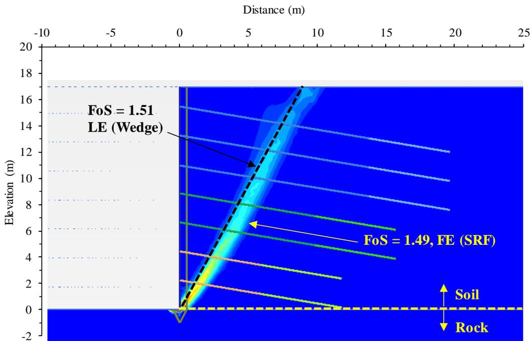
**Figure 4-79: Comparable failure mechanism for FE (SRF) and Wedge Method for rock below toe using anchor working load**
