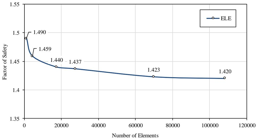
**Figure 4-10: FoS against number of elements for a global mesh size**
