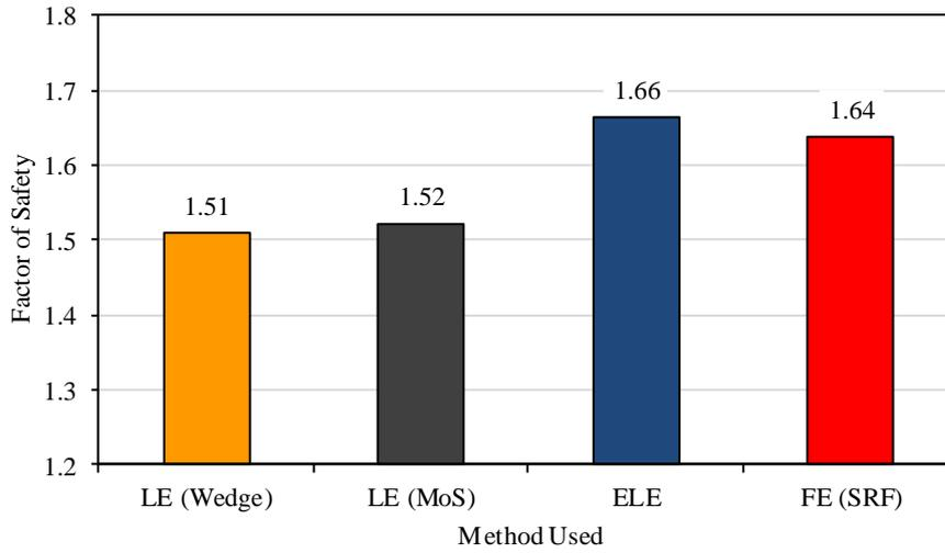
Figure 4-39: Minimum FoS obtained from various methods for anchored excavation
