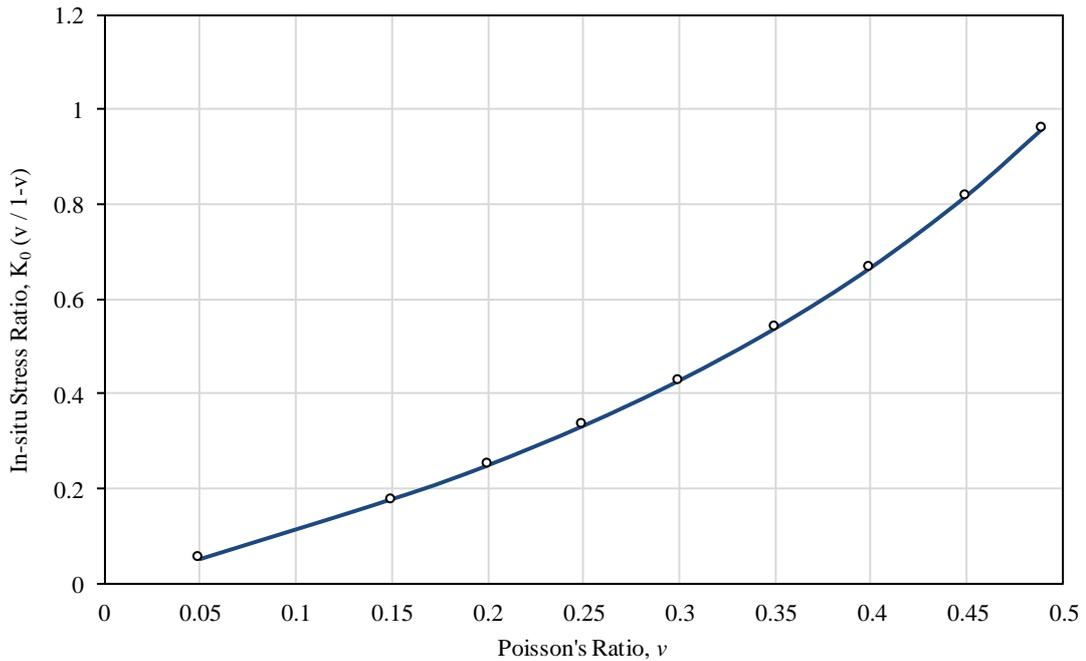
**Figure 4-23: In-situ stress ratio,  $K_0$ , values for specified Poisson,  $\nu'$ , using 1-Dimensional compression**
