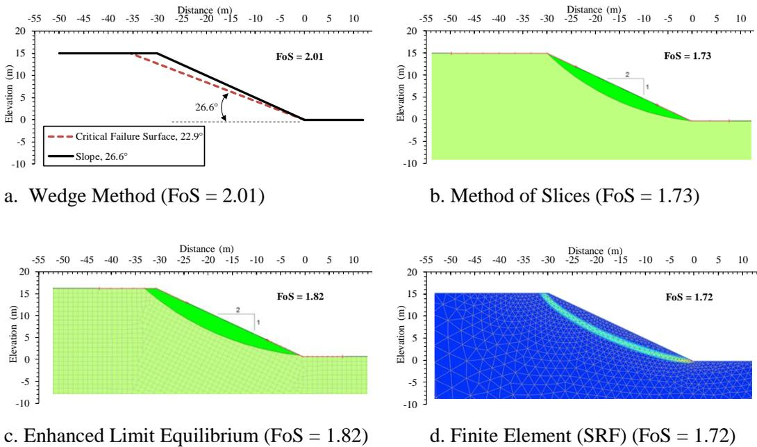
**Figure 4-2: Uniform slope critical failure mechanisms and associated factors of safety**
