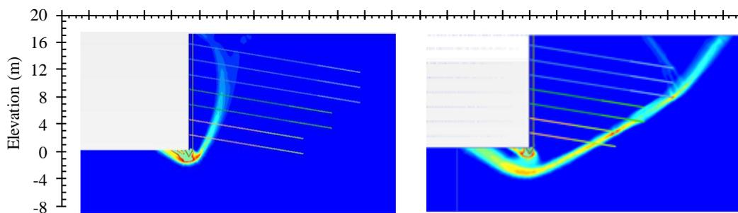
**Figure 4-58: Failure Mechanisms (left – *yielding*; right – *global*)**
