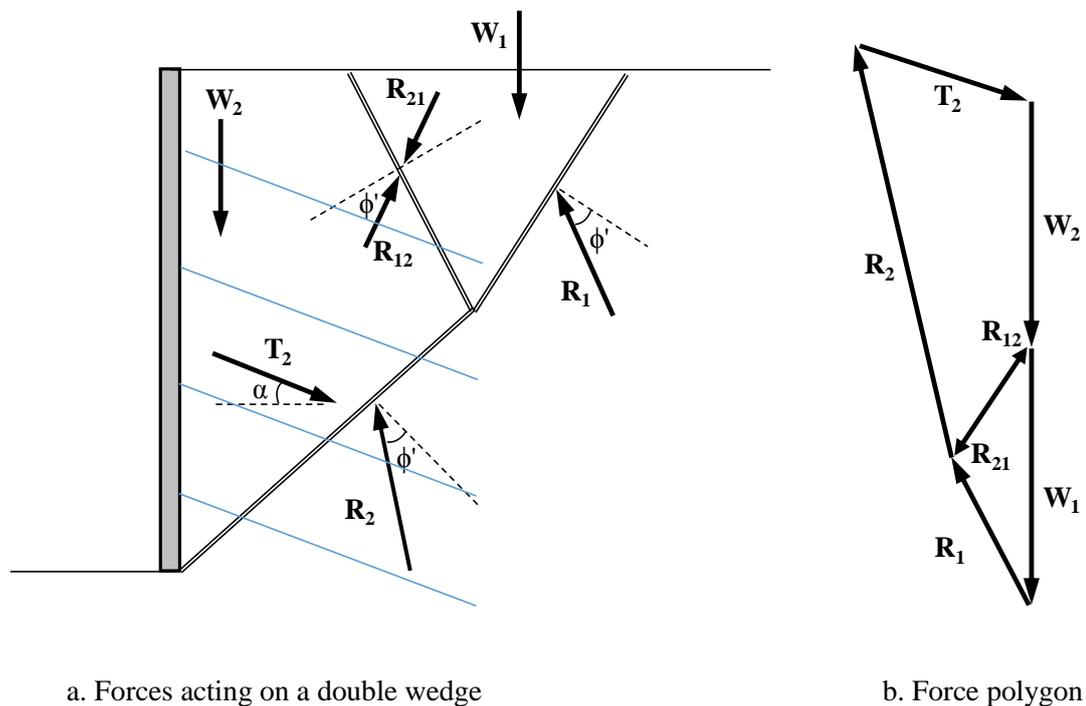
**Figure 2-26: Double trial wedge method**
