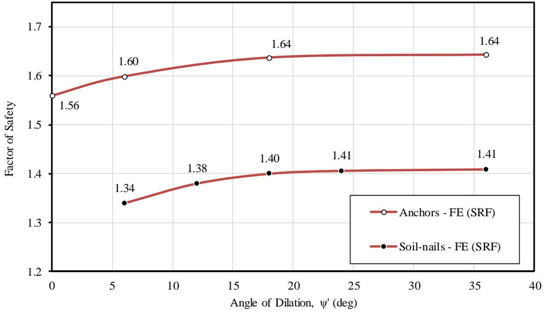
**Figure 4-80: FoS against angle of dilation for soil-nailed and anchored excavations for FE (SRF) Method**
