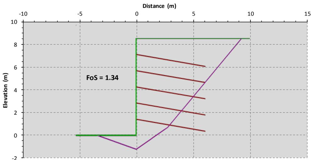
**Figure 4-74: Multiple wedge analysis critical FoS and compound failure mechanism**
