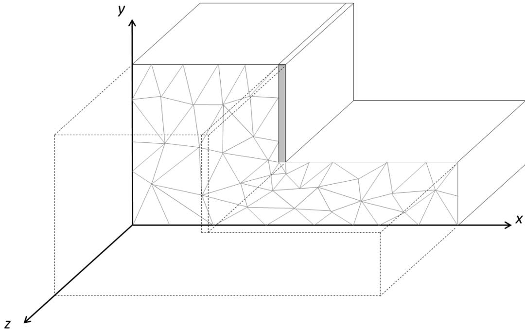
**Figure 2-36: Example of plane strain analysis (adapted from PLAXIS, 2016)**
