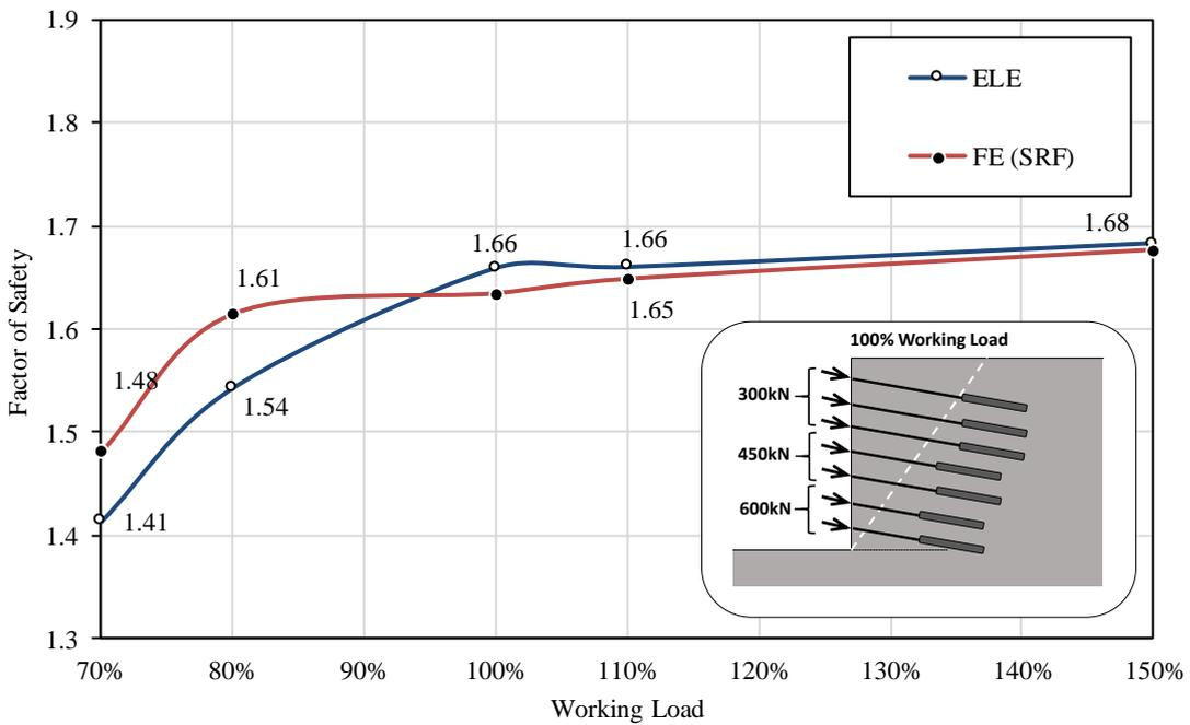
**Figure 4-60: FoS for a change in anchor working load for ELE and FE (SRF) Methods**
