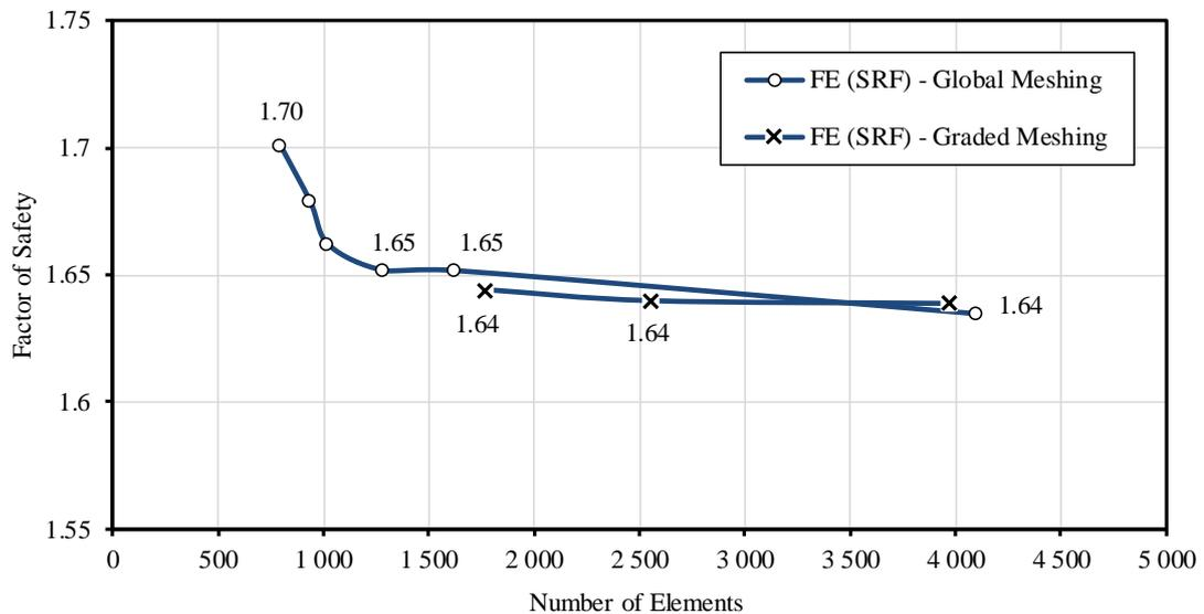
**Figure 4-43: FoS against number of elements for a global mesh size versus graded meshing for FE (SRF) model**
