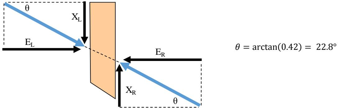
**Figure 2-30: Angle of interslice result force**
