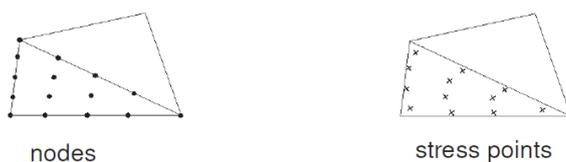
**Figure 2-37: Fifteen-noded triangular elements**
