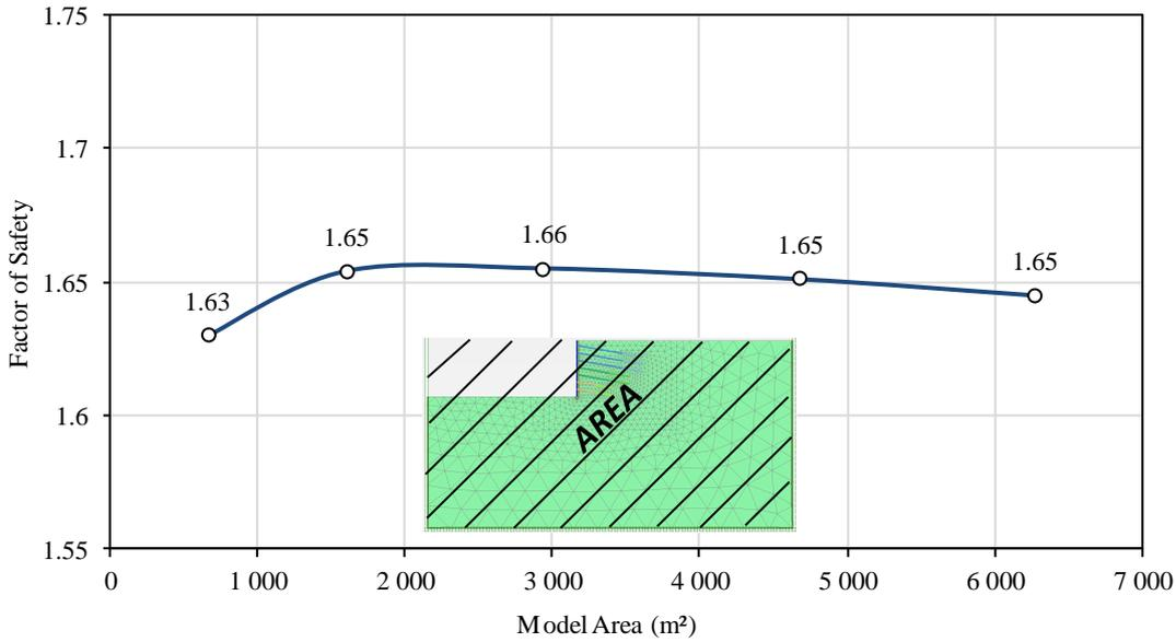
**Figure 4-44: FoS as function of the model cross-sectional area**
