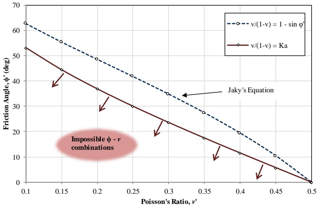
Figure 4-72: Possible and impossible  $\phi'$ - $\nu'$  combinations for Rankine's active and Jaky (1944) against 1-D compression
