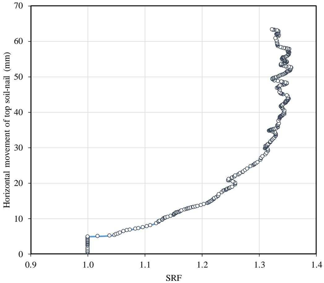
**Figure 4-81: Movement of lateral support against SRF for soil-nailed excavation using  $\psi' = 6^\circ$**
