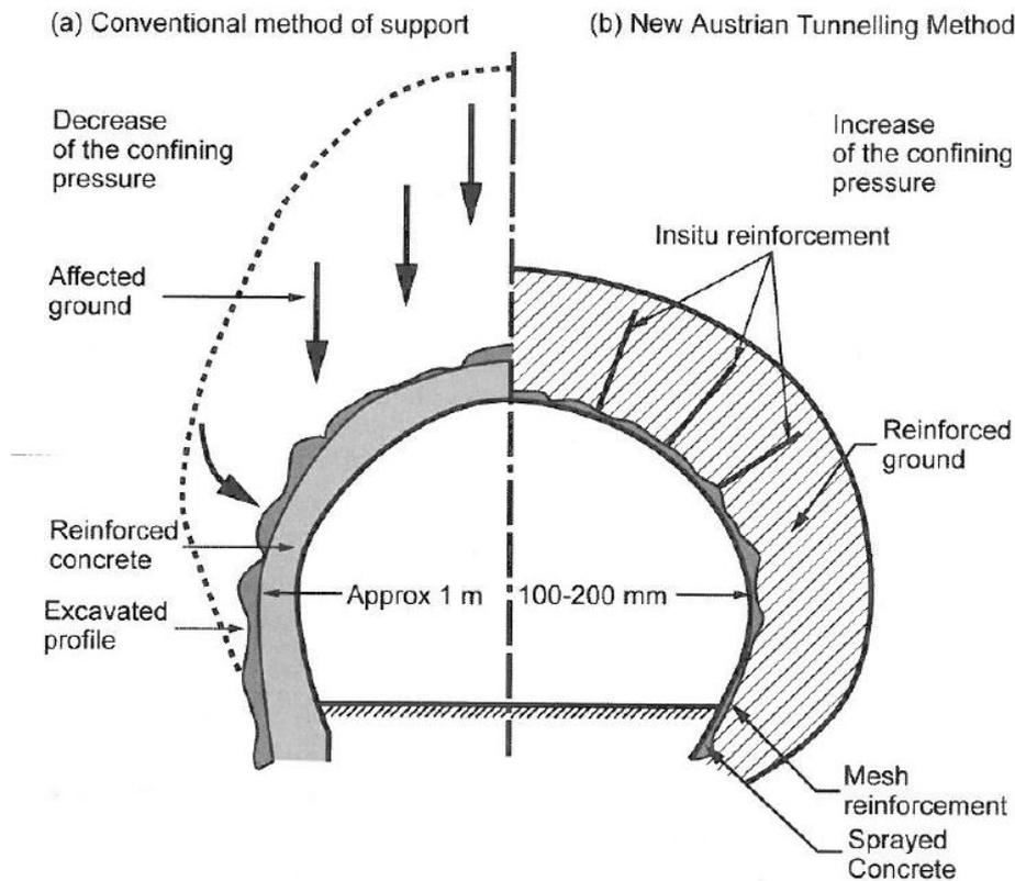
**Figure 2-1: Comparison of conventional supported arches and New Austrian Tunnelling Method (Bruce & Jewell, 1987)**
