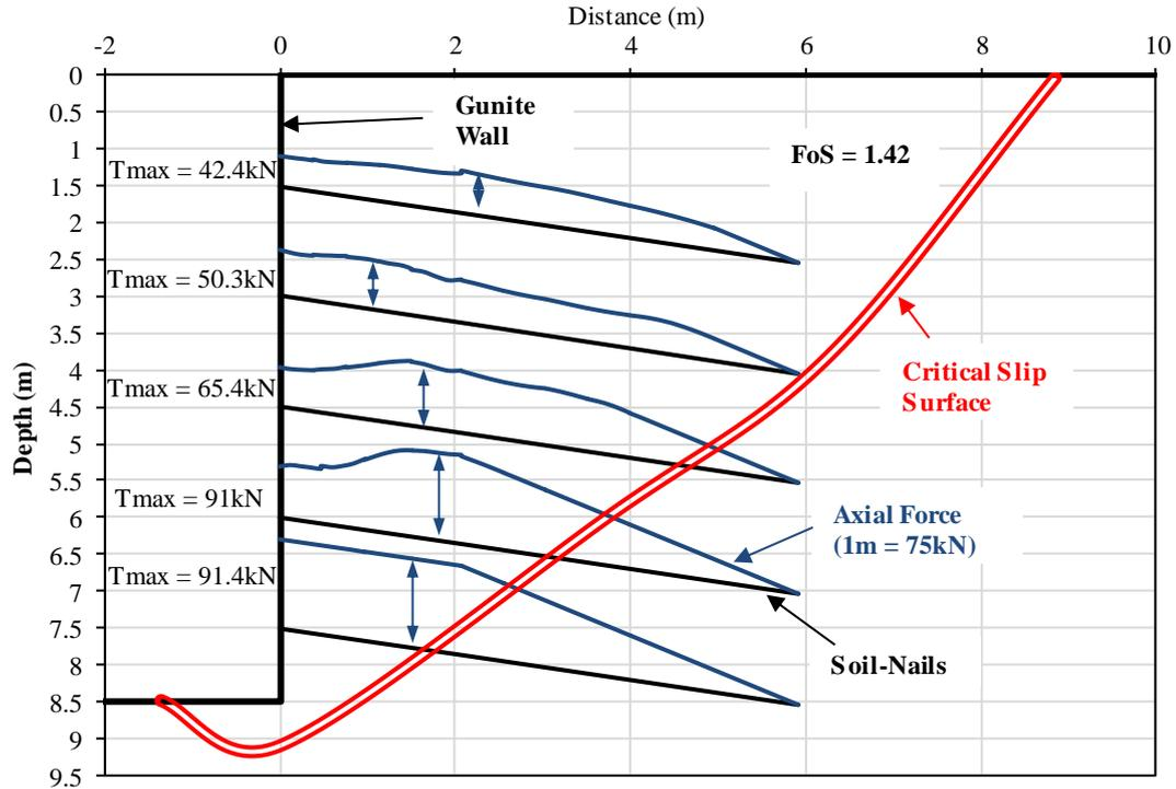
**Figure 4-32: FE (SRF) Method – soil-nail axial force distribution**
