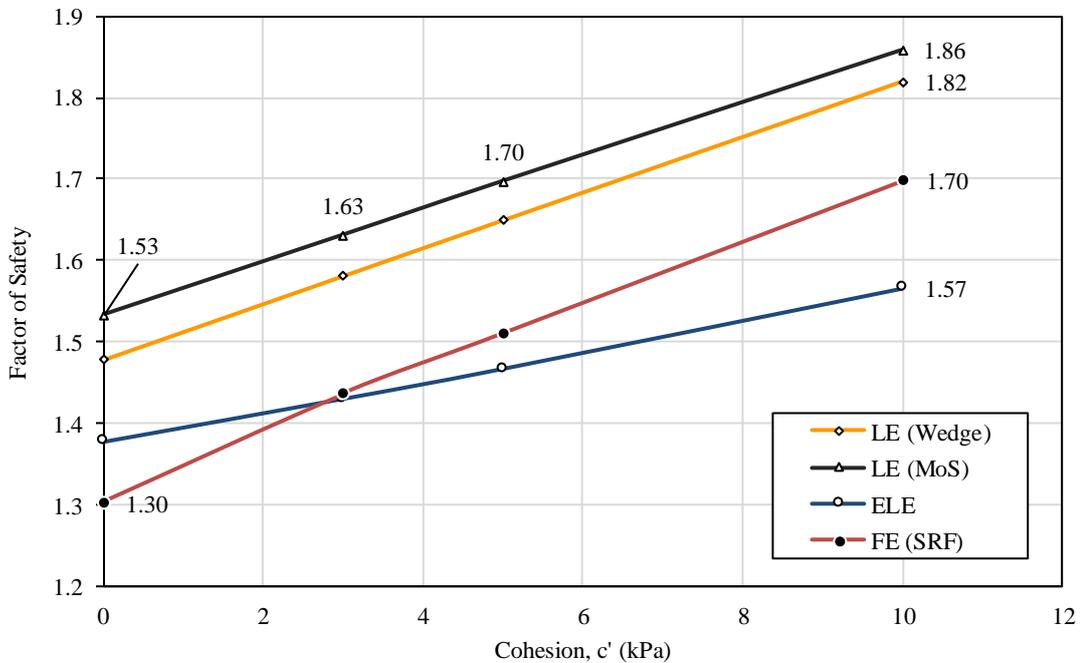
**Figure 4-19: FoS for a change in cohesion,  $c'$**
