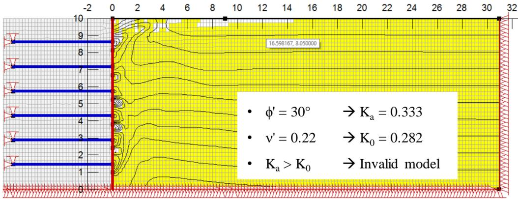
Figure 4-71: Cross-section of propped excavation showing in-situ stress violation
