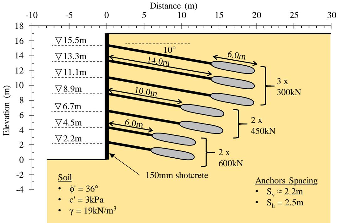
**Figure 3-3: Anchored excavation design**
