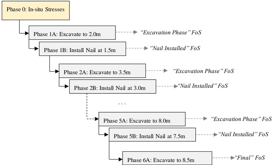
Figure 4-27: Construction sequence of soil-nailed excavation
