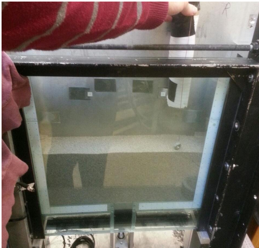
Figure 3-30: Sand being pluviated from a hopper into test frame
