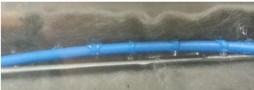
Figure 3-16: Perforated pipe on layer of Bidim, used to introduce moisture to the sample
