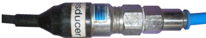
Figure 3-12: Pressure transducer (from O'Brien, 2013)
