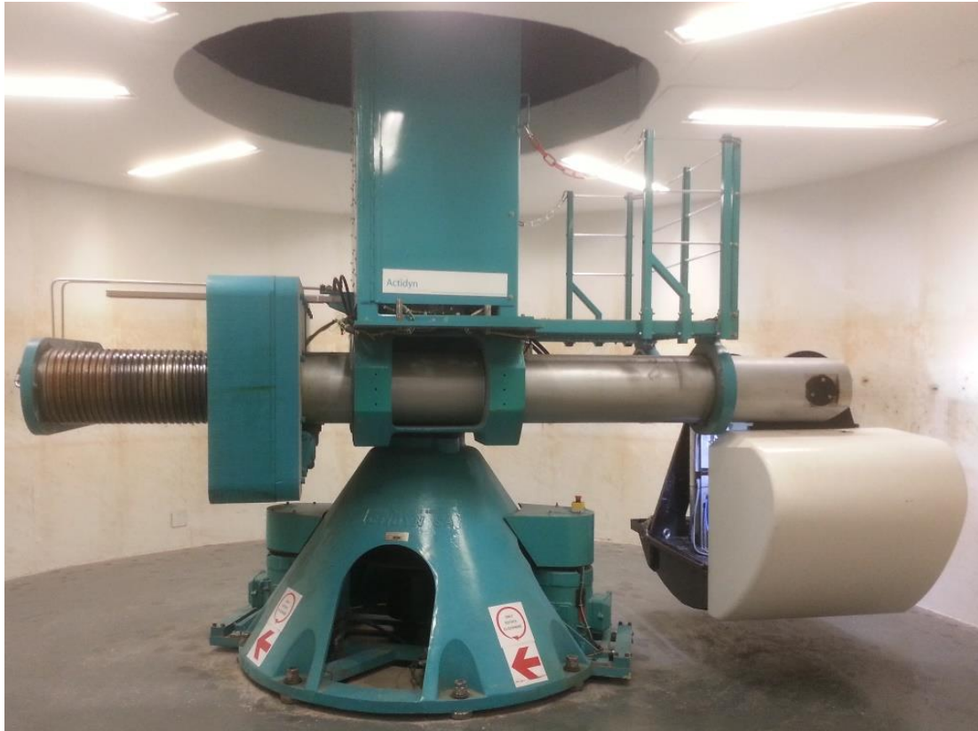
Figure 3-2: Geotechnical centrifuge at the University of Pretoria
