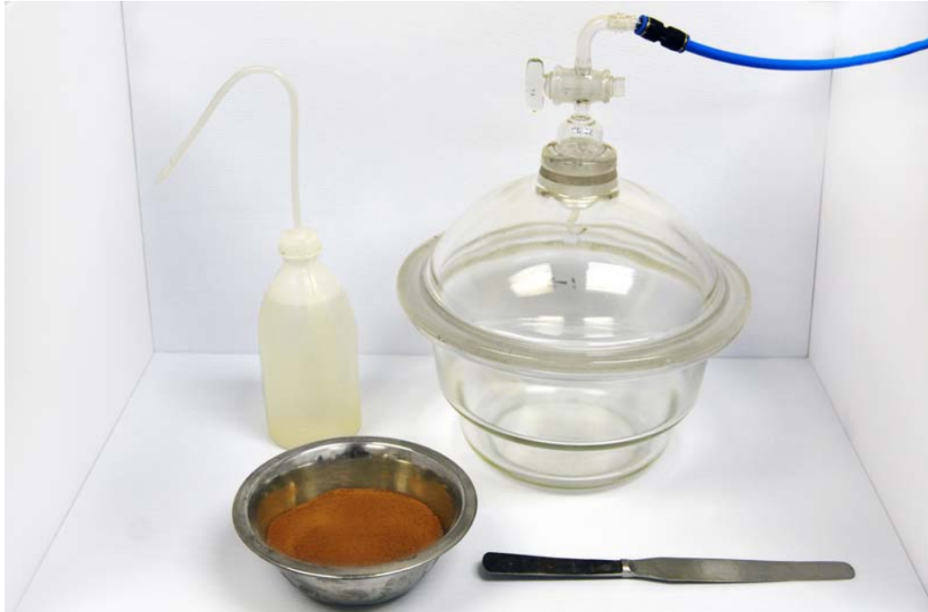
Figure 4-10 Equipment for mixing of soil specimen
