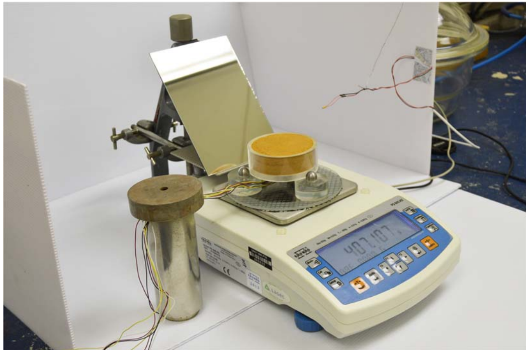
Figure 4-8 Continuous drying test setup during testing
