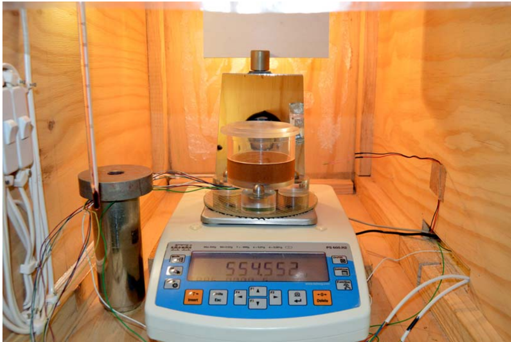
Figure 4-12 Continuous drying test setup in the enclosure
