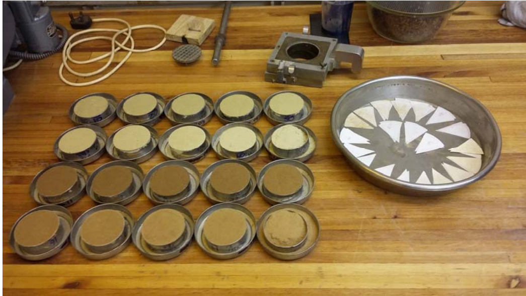
Figure 4-17 Filter paper specimens after oven-drying
