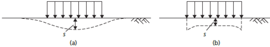
Figure 2-12: Distribution of vertical displacement beneath a flexible area: (a) clay and (b) sand (Knappett and Craig, 2012)
