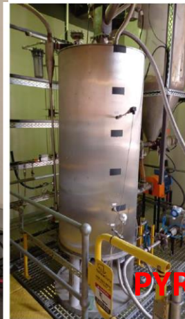
Pyrolyser(front), feed bin(behind), blower(back right) Separation equipment (left back)
