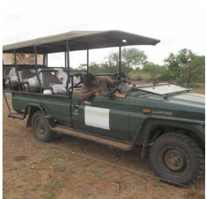
A game drive vehicle loaded with 10 sand bags, each weighing 70 kg, was used to simulate conditions in which a vehicle, fully laden with tourists (weighing about 3 795 kg in total) will drive in different conditions.
