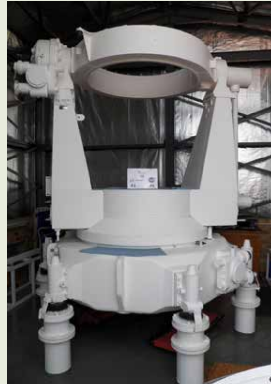
Actual representation of the external metallic structure of the LLR telescope at HartRAO.
