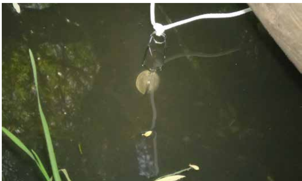
The low cost sampler collecting pollutants in the Hartbeesspruit
