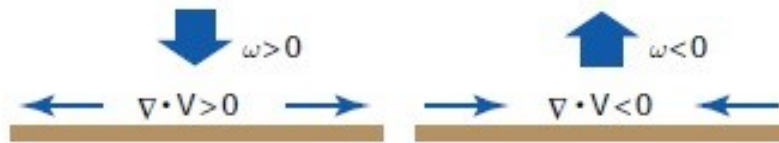
Figure 5: Algebraic signs of \omega in the midtroposphere associated with convergence and divergence in the lower troposphere. [Source: Wallace, J.M. and Hobbs, P.V. (2006). Atmospheric Science: An Introductory Survey, 2nd Ed. Academic Press, pp. 483]
