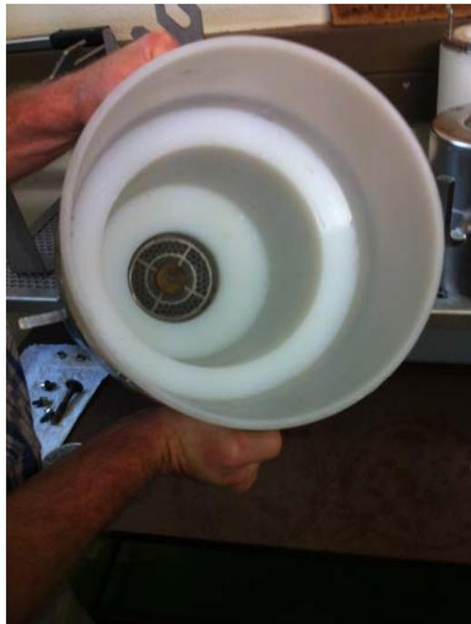
Remove the assembly from the jig and, after rechecking all parts are correctly assembled, fill the assembly partially with water. Then squeeze and pump the rubber sample receptacle at the base of the assembly to remove all air bubbles. Open the Selfrag doors and place the assembly in the Selfrag, ensuring that the assembly fits firmly into the fitting mounts in the green base of the device.
