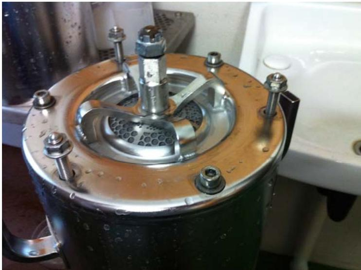
Place the assembly in the assembly jig. Fit the pre-cleaned black rubber mineral collection receptacle in its metal holder, attach both to the base of the metal polypropylene assembly (within the jig) and, ensuring it is in the correct orientation, tighten the 3 retaining nuts to the correct tension.
