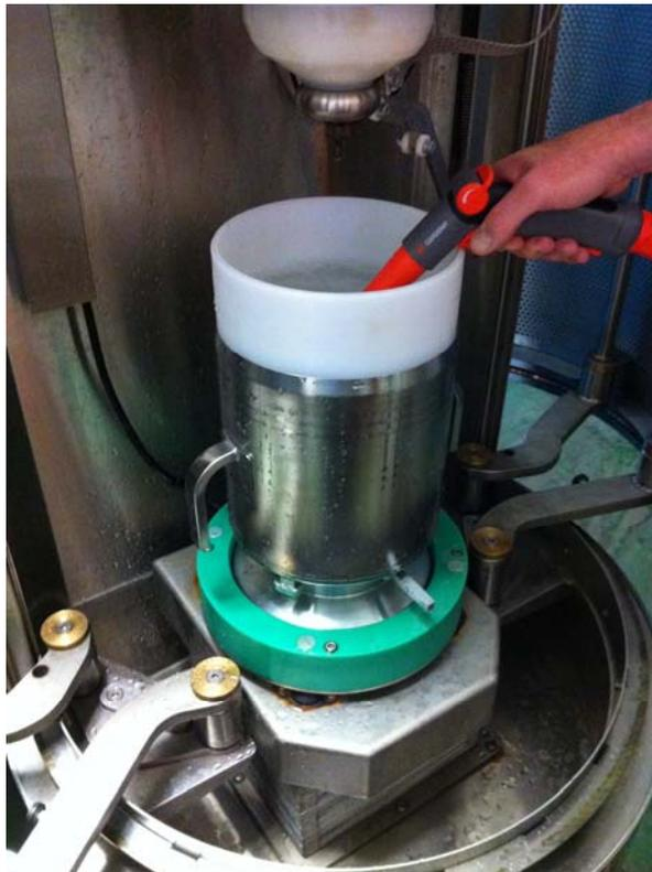
The instrument is now ready for calibration of the electrode gap. On the instrument panel, run the “Calibration of the Electrode Gap” routine. On completion, open the instrument doors and remove the Calibration Spacer from the sample receptacle.
