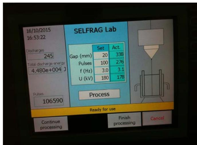
Close the instrument doors. Set the gap initially to 30 mm, pulses to 100, Frequency to 3.0 and kV to 180 and start the processing routine.
