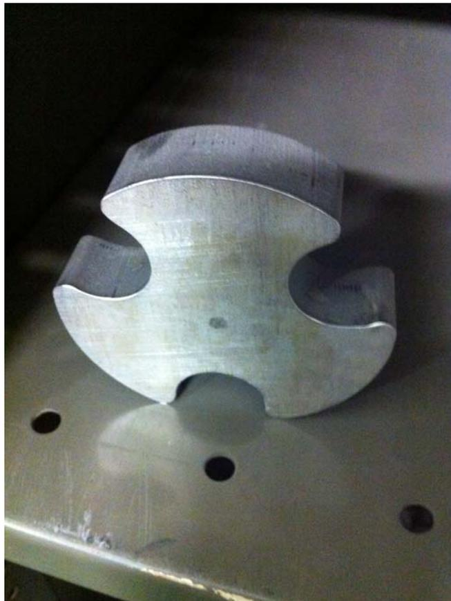
Place the pre-cleaned Calibration Spacer (see above) into the sample assembly and further fill the sample assembly with water to the top of the bevel in the polypropylene container. Close the instrument doors.
