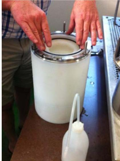
As the fragmentation process generates significant vibration that can cause nuts to loosen, ensure that all nuts during assembly are tightened on bolts to the tension specified by the manufacturer using a torque wrench.
