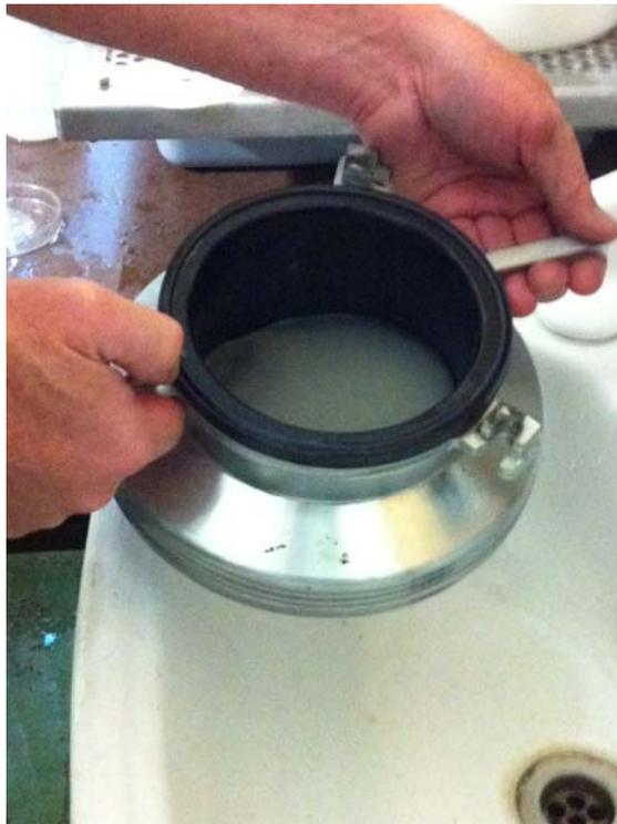
When sufficient material has passed through the mesh and processing is completed, remove the assembly and dismantle the base, containing the rubber sample receptacle. Decant off the excess water. Rounded metal particles derived from the electrodes will also be present in the sample and should be removed using a hand magnet when processing is complete.
