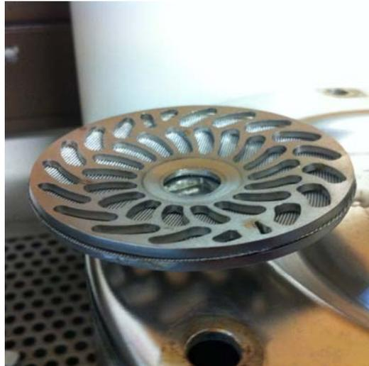
Assemble the mesh into the mesh holder and pass the electrode bolt through the mesh assembly.
