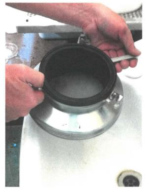
When sufficient material has passed through the mesh and processing is completed, remove the assembly and dismantle the base, containing the rubber sample receptacle. Decant off the excess water. Rounded metal particles derived from the electrodes will also be present in the sample and should be removed using a hand magnet when processing is complete.
