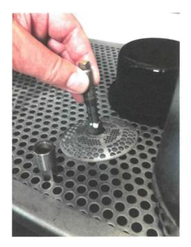
Assemble the polypropylene container into the metal sleeve with the O-rings intact, ensuring that the 3 retaining bolts are tightened to the correct tightness using a torque wrench. Pass the electrode bolt with mesh holder through the polypropylene container and attach it to the metal sleeve using the nut provided. Tighten to the correct tightness using a torque wrench. Fit the spacer bolt to the protruding end of the electrode and tighten to the correct tension using a torque wrench.
