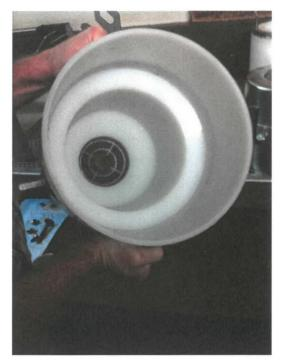
Remove the assembly from the jig and, after rechecking all parts are correctly assembled, fill the assembly partially with water. Then squeeze and pump the rubber sample receptacle at the base of the assembly to remove all air bubbles. Open the Selfrag doors and place the assembly in the Selfrag, ensuring that the assembly fits firmly into the fitting mounts in the green base of the device.
