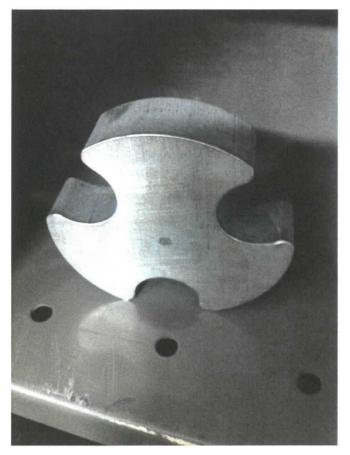
Place the pre-cleaned Calibration Spacer (see above) into the sample assembly and further fill the sample assembly with water to the top of the bevel in the polypropylene container. Close the instrument doors.
