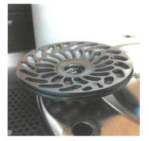
Assemble the mesh into the mesh holder and pass the electrode bolt through the mesh assembly.
