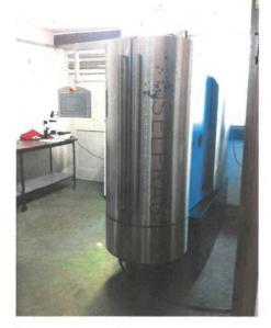
To begin sample fragmentation, turn on the Selfrag instrument using the power switch (right hand side of instrument) and open the  $N_2$  gas supply valve to the instrument. On the control panel, log in to the instrument and allow it to complete its self-test procedure.
