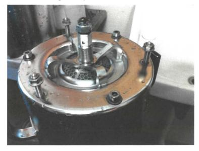
Place the assembly in the assembly jig. Fit the pre-cleaned black rubber mineral collection receptacle in its metal holder, attach both to the base of the metal polypropylene assembly (within the jig) and, ensuring it is in the correct orientation, tighten the 3 retaining nuts to the correct tension.
