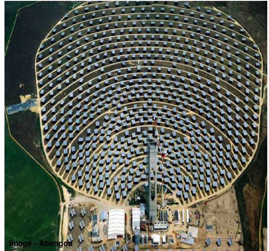
Single sided field – cavity receiver
