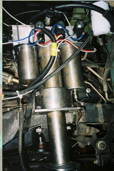
Computerised hydro-pneumatic suspension system (2007 - )
