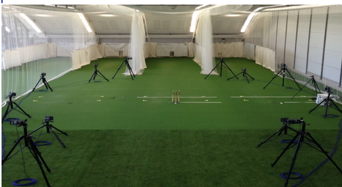
Three-dimensional motion capture setup in the Cricket South Africa Centre of Excellence at the University of Pretoria
