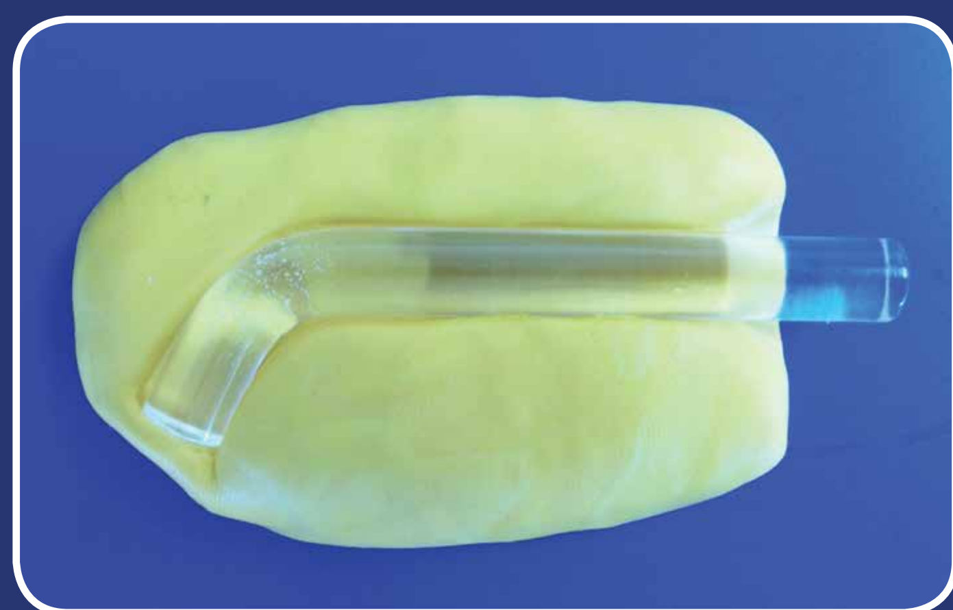
Figure 1: 10 cm acrylic rod (8 mm in diameter), shaped into a 145 degree angle.
