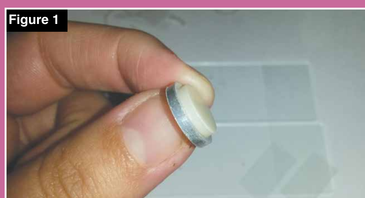
Figure 1 Composite sample being removed from the ring mould, after being cured between two glass plates under a Mylar strip.
