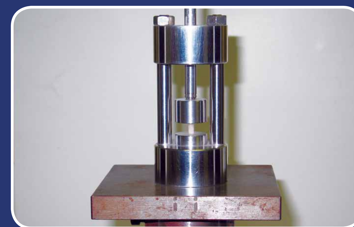
Figure 3: Instron machine with composite specimen mounted into Bencor Multi-T device.
