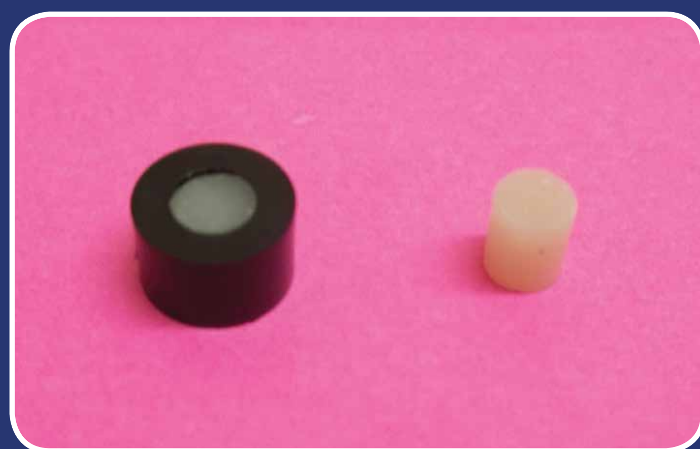
Figure 2: Composite specimens packed into Teflon moulds.
