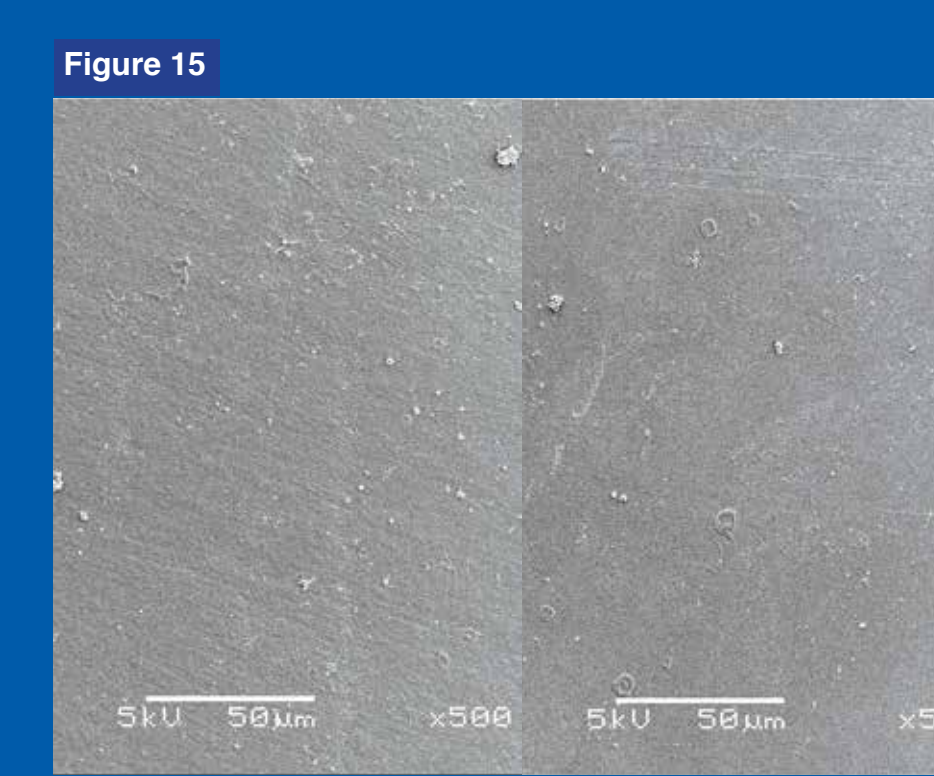
Figure 15 Right: Filtek™ Supreme XTE polished with Sof-lex™ Spiral Wheels followed by Zircon-Brite. The surface is very smooth, with protruding filler particles of different sizes visible.
