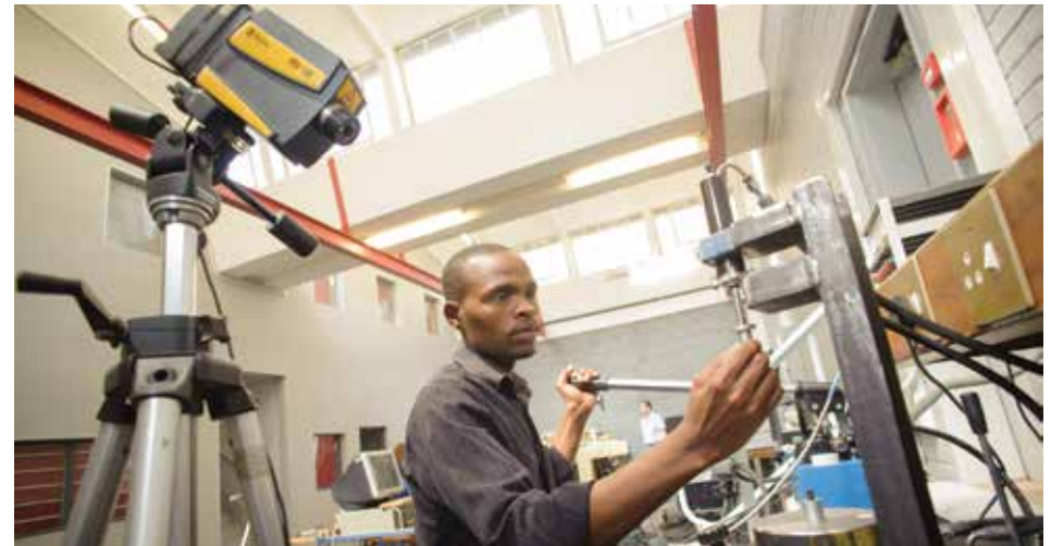
Structural dynamics testing using non-contact optical measurements
