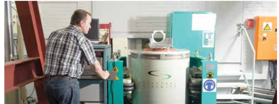
Durability testing using large electrodynamic actuator
