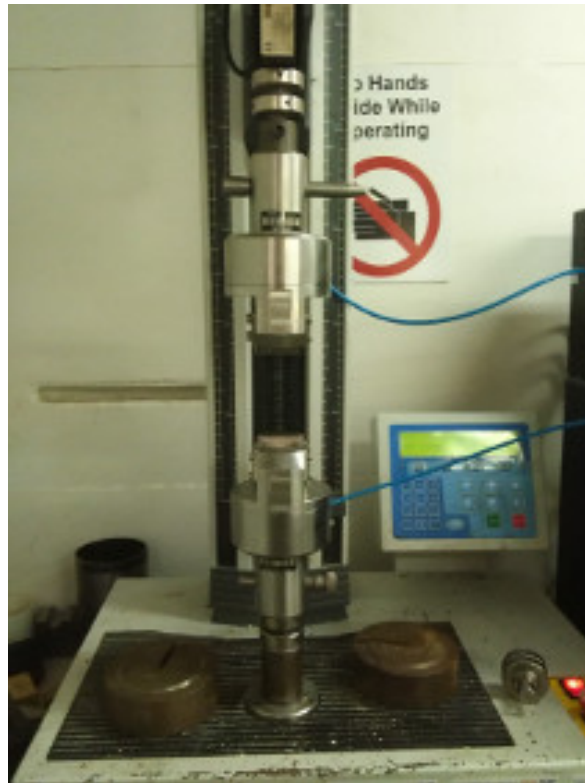
Figure 5.10: Tensile testing of the HaTe ® mesh with a 5 kN Lloyd's Tensile Tester.
