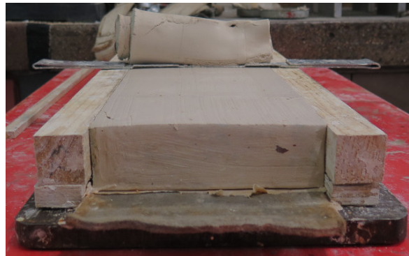
Figure 3.11: Trimming the consolidated clay liner to the required thickness.
