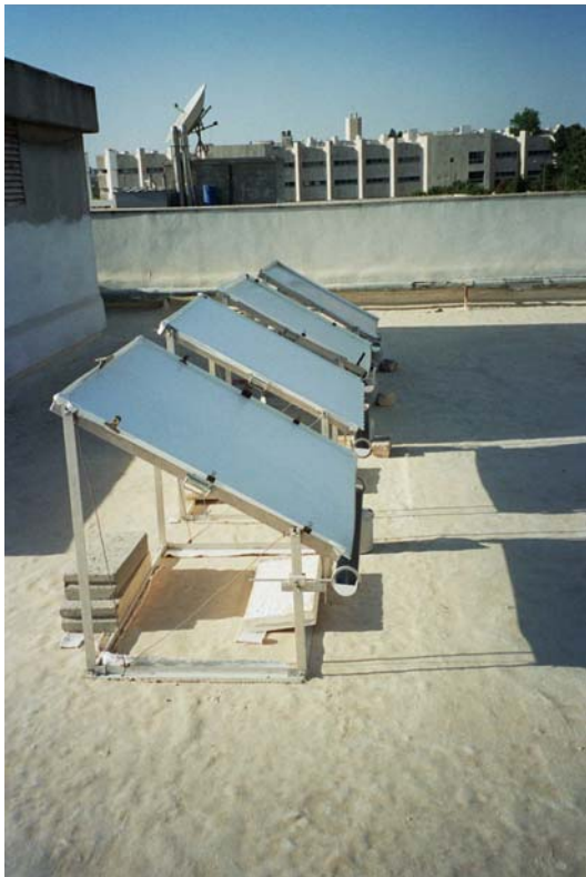
Figure 1: View of the rooftop dew collector setup in Jerusalem.
